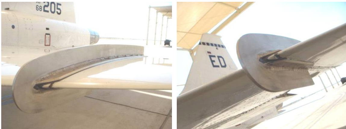
Figure 62. Top and Bottom Photographs of the Installed Left Wing Fence (36)
