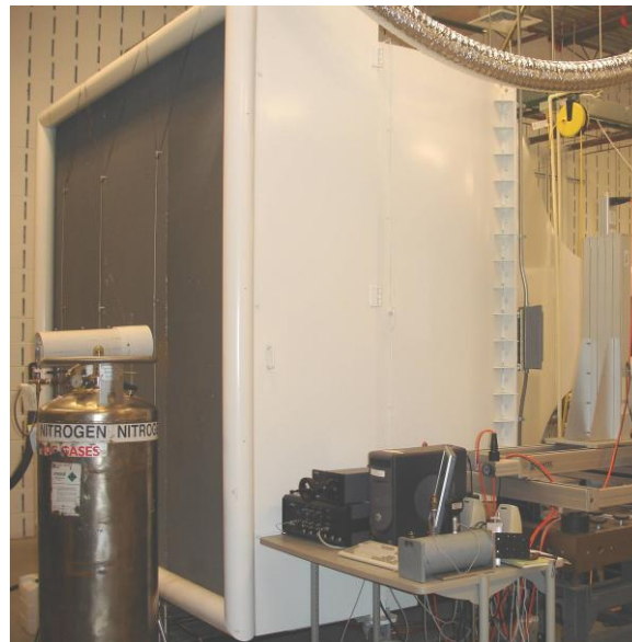
Figure 49. Intake and Convergent Section of the Wind Tunnel
