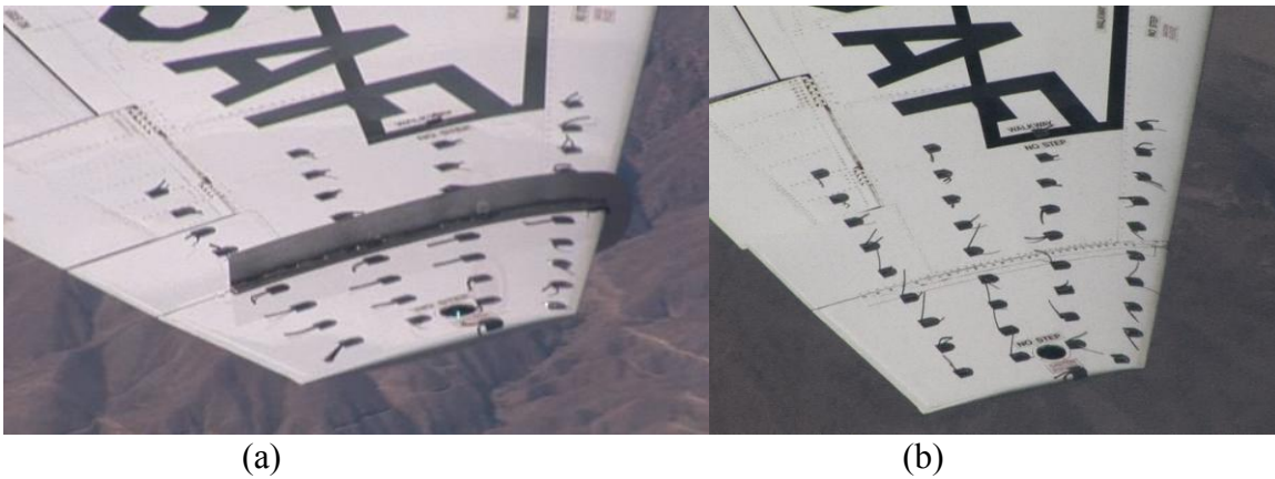
Figure 141. Fence and Clean Tufted Wings at 14.9 degrees AOA (1.0 normalized) (a) 153 KCAS (b) 152 KCAS
