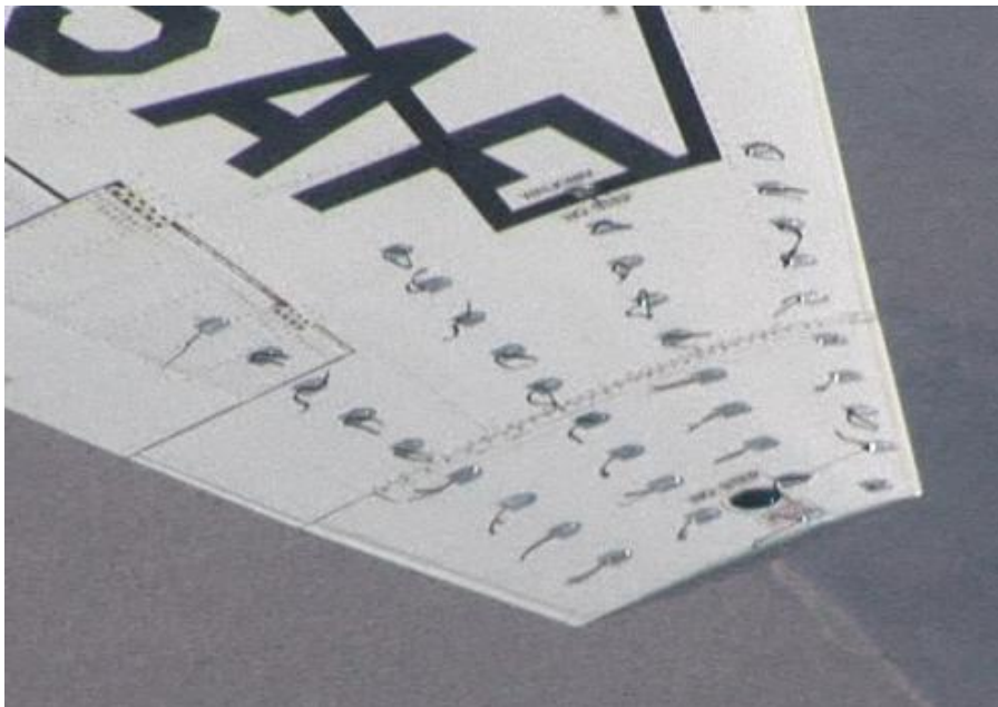
Figure 179. Clean Tufted Wing at 9.3^\circ AOA (0.63 normalized) and 185 KCAS
