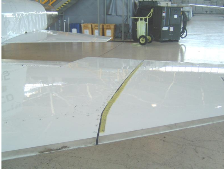
Figure 4. T-38 Wing Seam Located 26.5 Inches from Wingtip
