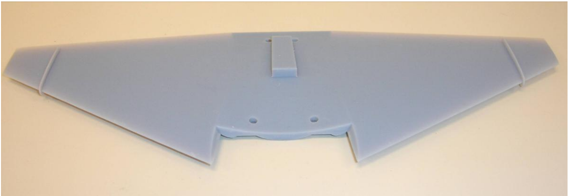
Figure 30. Top View Model Wing Fence
