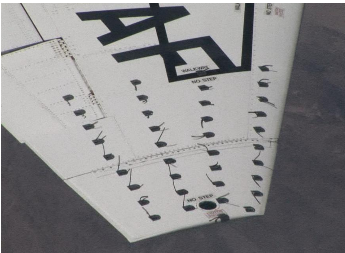
Figure 205. Clean Tufted Wing at 14.9^\circ (1.0 normalized) AOA and 152 KCAS
