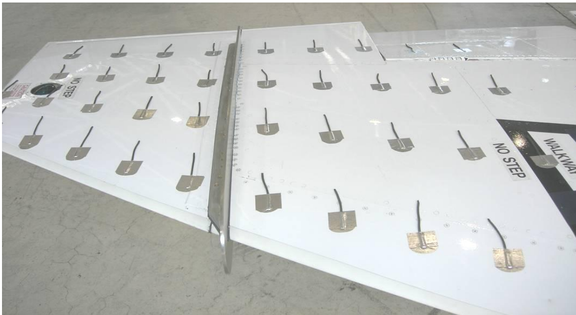
Figure 65. Flight Test Installed Tufts (Front View)
