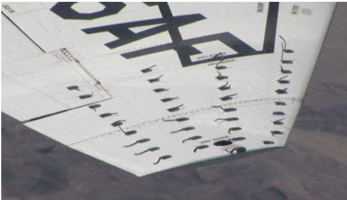
Figure 197. Clean Tufted Wing at 12.4^\circ AOA (0.83 normalized) and 156 KCAS
