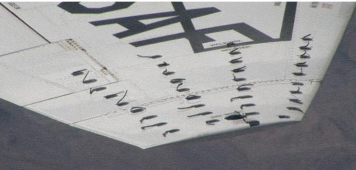
Figure 177. Clean Tufted Wing at 8.6^\circ AOA (0.58 normalized) and 183 KCAS
