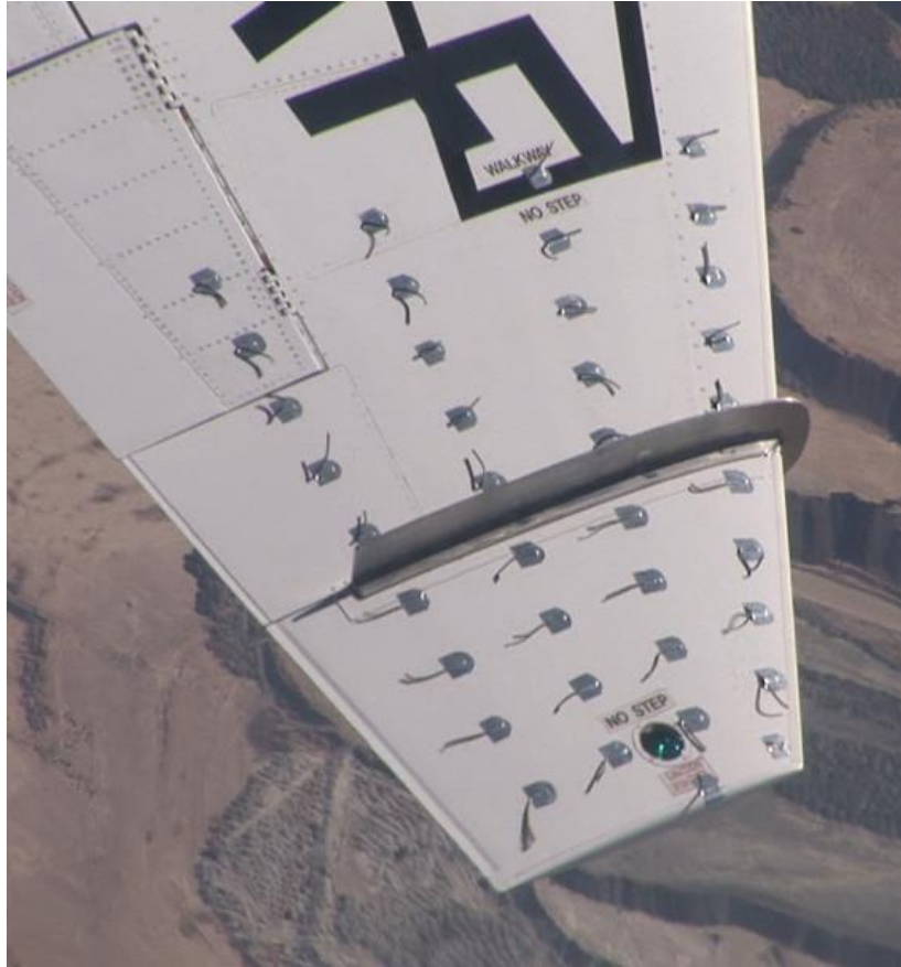
Figure 192. Fence Tufted Wings at 11.9^\circ AOA (0.80 normalized) and 151 KCAS
