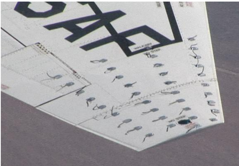
Figure 181. Clean Tufted Wing at 9.5^\circ AOA (0.64 normalized) and 179 KCAS
