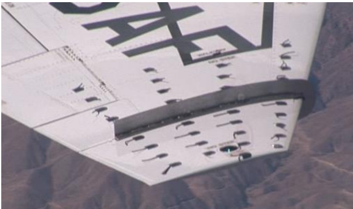
Figure 204. Fence Tufted Wings at 14.9^\circ (1.0 normalized) AOA and 153 KCAS
