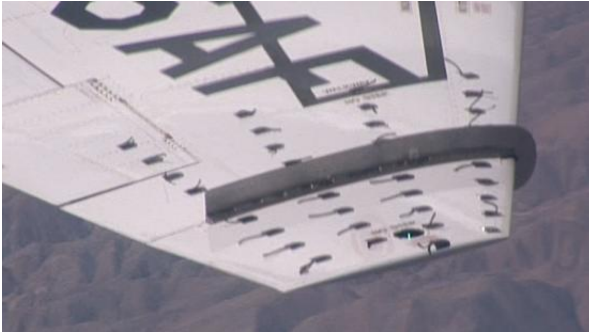
Figure 196. Fence Tufted Wings at 12.4^\circ AOA (0.83 normalized) and 154 KCAS
