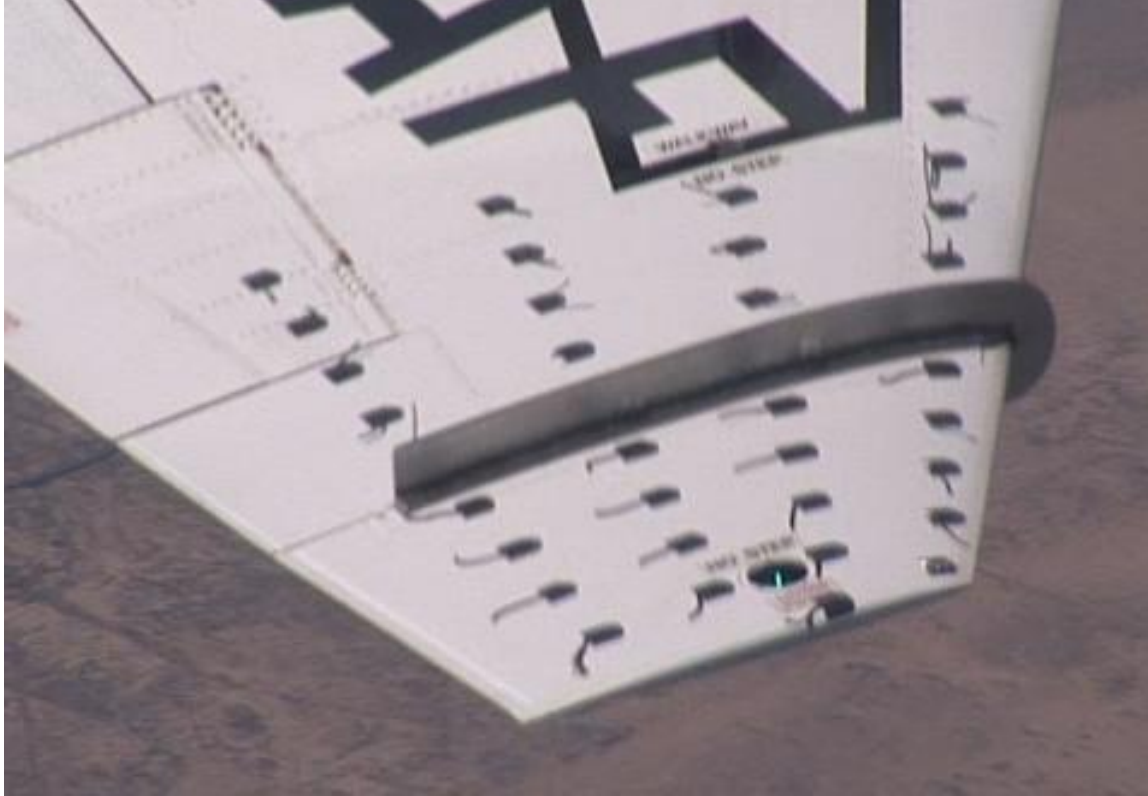
Figure 182. Fence Tufted Wing at 9.6^\circ AOA (0.65 normalized) and 174 KIAS
