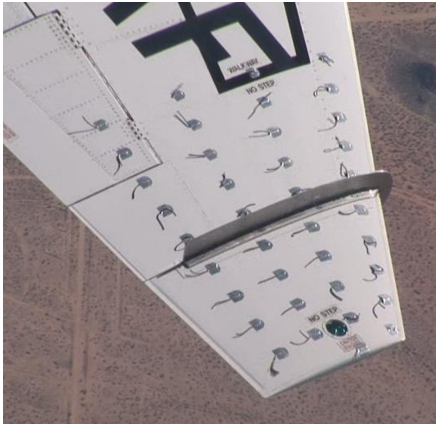
Figure 178. Fence Tufted Wing at 9.3^\circ AOA (0.63 normalized) and 168 KCAS
