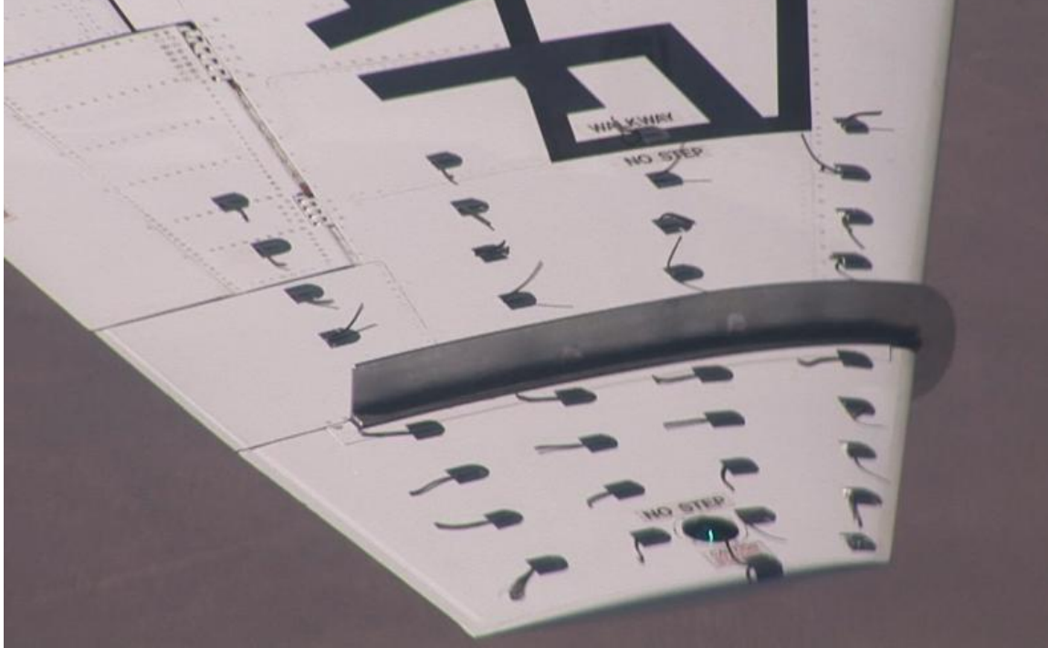
Figure 202. Fence Tufted Wing at 14.2^\circ AOA (0.94 normalized) and 146 KCAS
