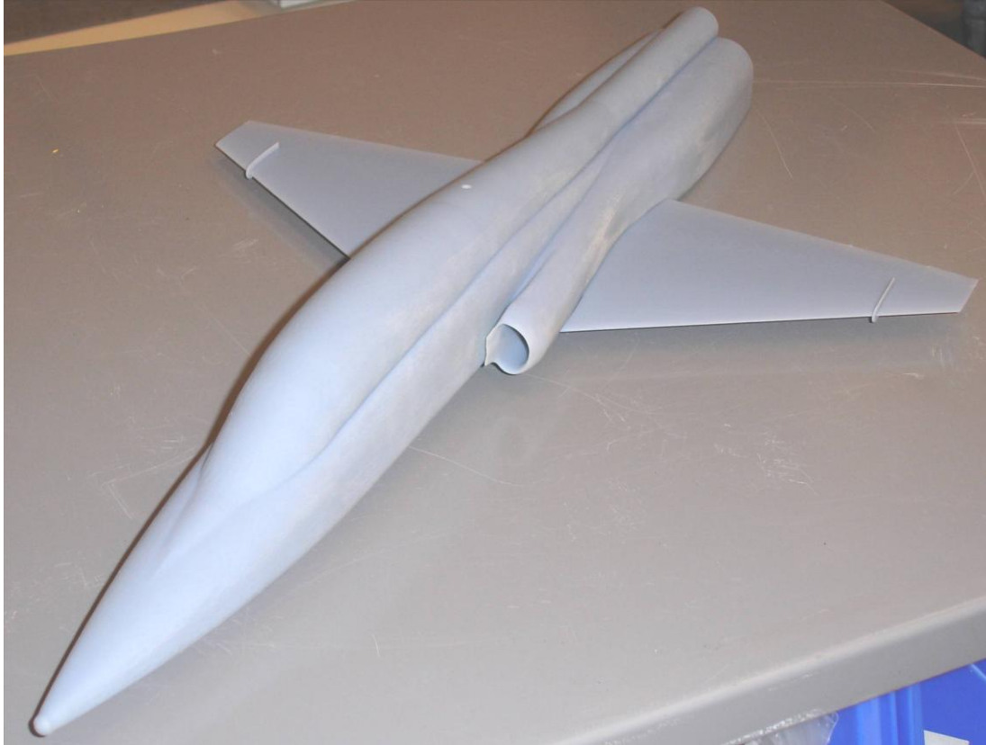
Figure 5. Photograph of T-38 Wind Tunnel Model with a Test Fence Installed
