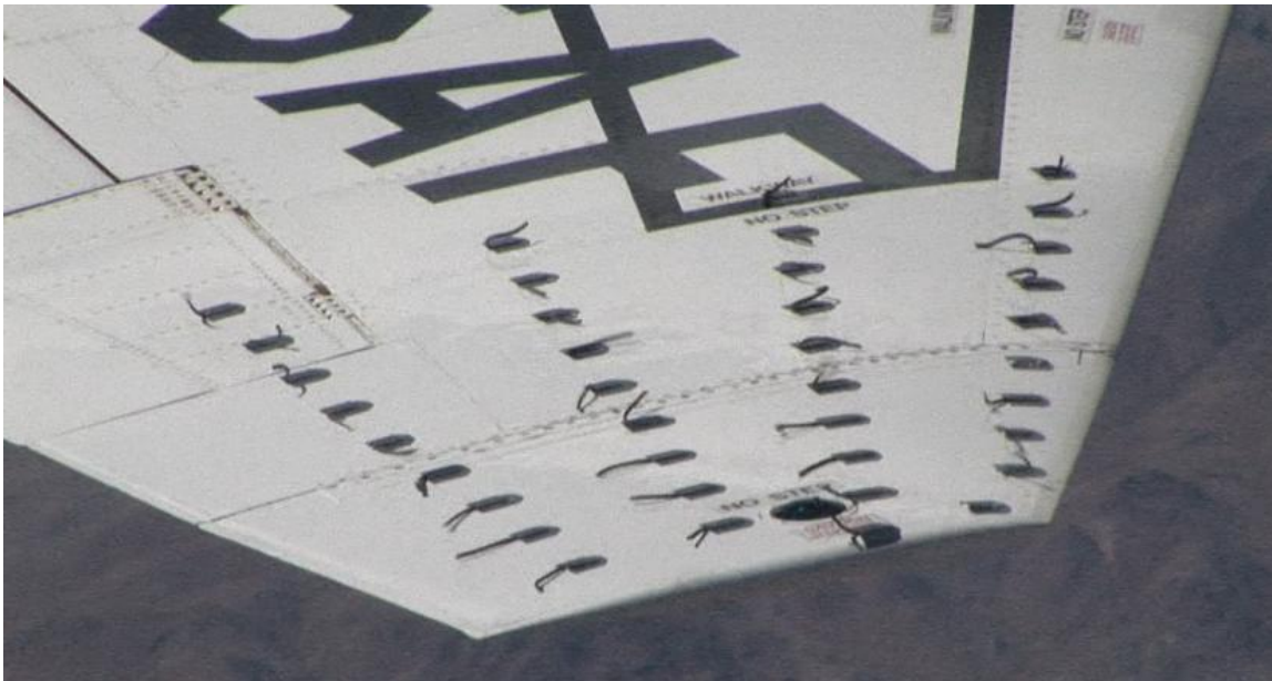
Figure 183. Clean Tufted Wing at 9.6^\circ AOA (0.65 normalized) and 175 KCAS
