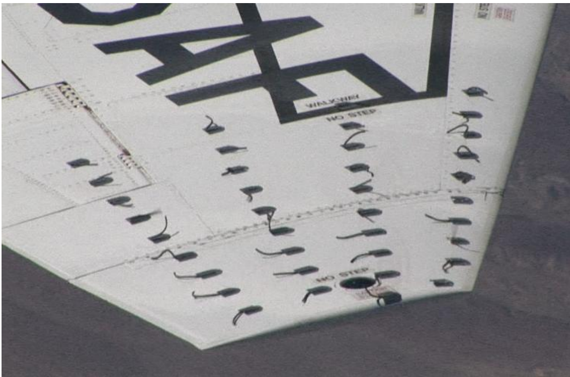
Figure 189. Clean Tufted Wing at 10.7^\circ AOA (0.72 normalized) and 165 KCAS
