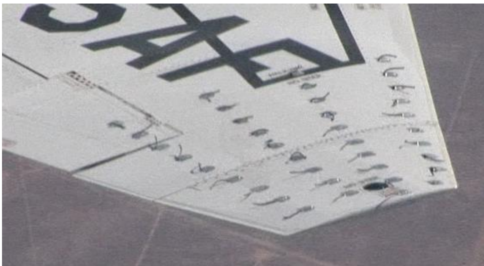
Figure 199. Clean Tufted Wing at 13.4^\circ AOA (0.90 normalized) and 153 KCAS
