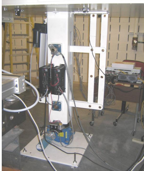
Figure 51. Sting Angle Control Device (13)
