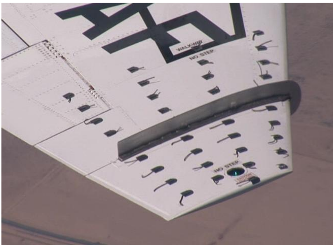
Figure 190. Fence Tufted Wing at 11.4^\circ AOA (0.77 normalized) and 159 KCAS
