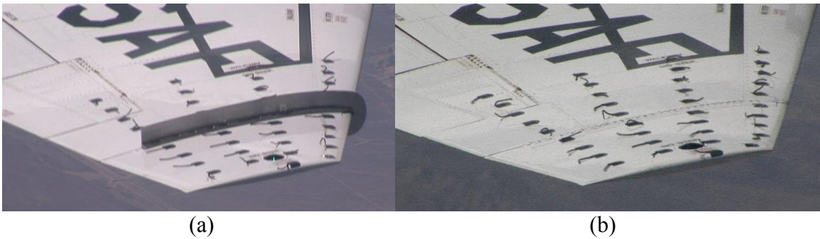
Figure 138. Fence and Clean Tufted Wings at 8.4 degrees AOA (0.56 normalized) (a) 185 KCAS (b) 188 KCAS
