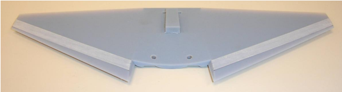
Figure 40. Model Clean Wing with Trip Tape (Top View)
