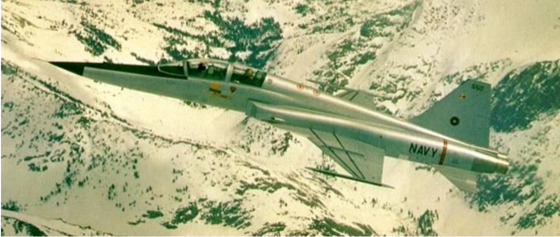
Figure 3. Navy F-5F with Wing Fences (Courtesy of Mr. Dennis Peters)
