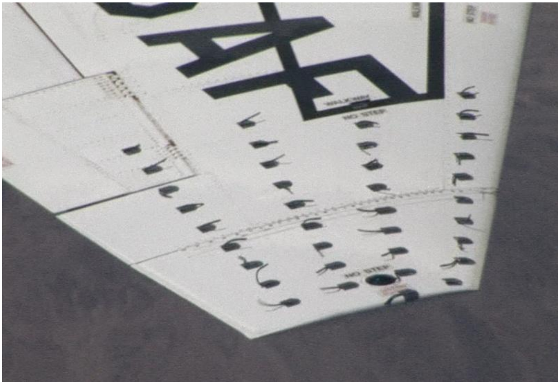
Figure 203. Clean Tufted Wing at 14.2^\circ AOA (0.94 normalized) and 152 KCAS
