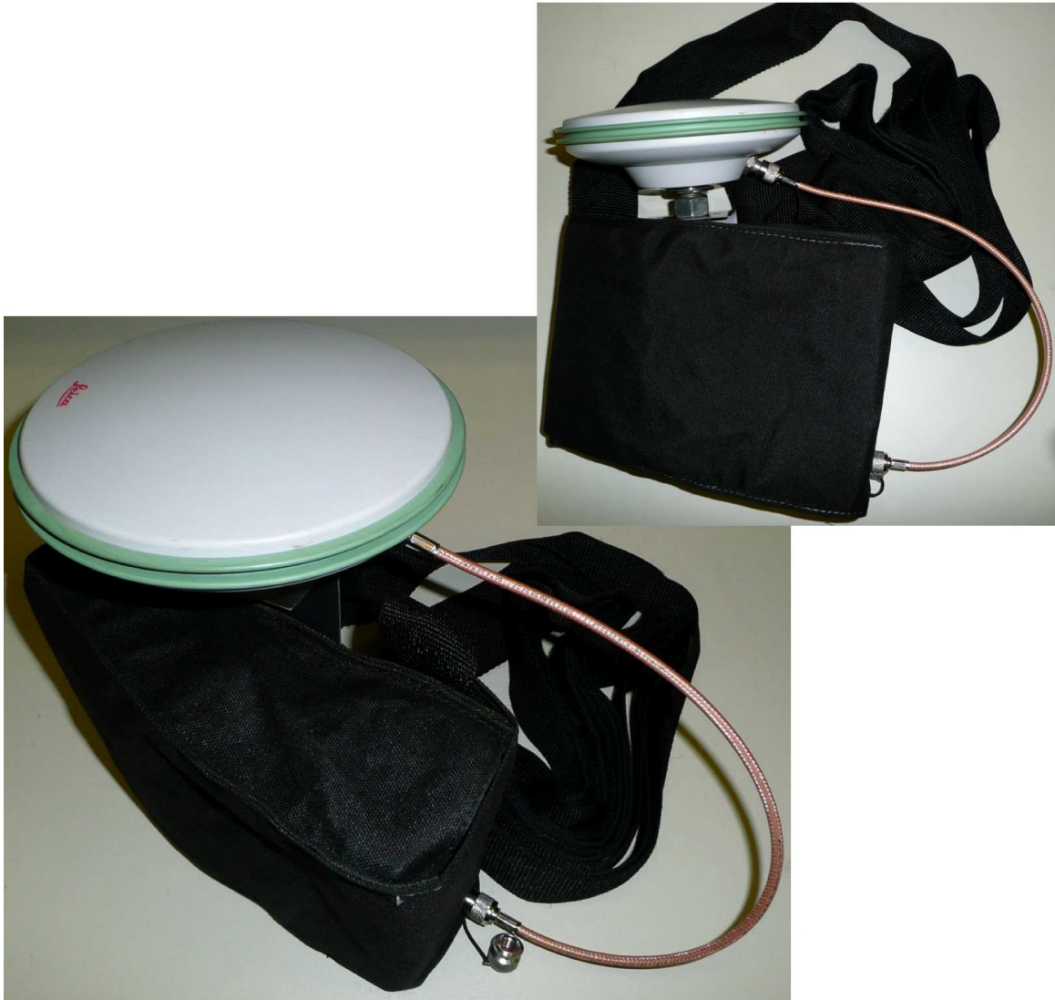
Figure 3.6: Nylon Pouch Made for Leica Recorder With Antenna Mount: Nylon webbing with velcro bands was used to lash the recorder to aircraft wingtip pylons. Pouches were made and provided by sailors of Strike Fighter Squadron Three Four - The Blue Blasters.
