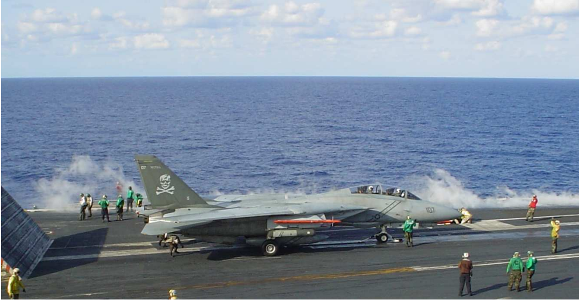
Figure 1.13: F-14 Tomcat Preparing for Launch: Of interest are two maintenance personnel immediately beneath the hot engine exhaust nozzles. Taken in 2004 by the author onboard USS John F. Kennedy (CV-67).
