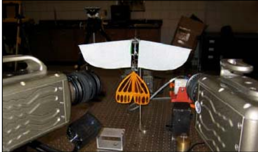
Figure 11: Visual Image Correlation Validation Set-Up (Stewart and Albertani, 2007)
