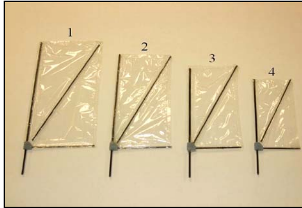
Figure 75: Carbon Fiber Framed and Mylar Membrane used by Svanberg (Svanberg, 2008)
