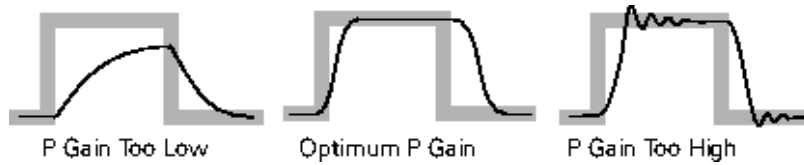
Figure 4.7: Effect of P Gain [56] on System Response
