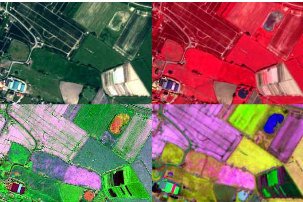
Left: Sub-image showing a true color composite (upper left), false color composite (upper right), pseudo color with red=Chlorophyll content, green=Leaf area index, blue=Average leaf angle (lower left) and pseudo color with red=Leaf area index, green=Structure coefficient, blue=Brown pigment (lower right). This image shows how different vegetation types can be distinguished using the false color images of the vegetation maps. A magenta colored path crossing the grassy area in the lower left center area is clearly visible in the lower right image, showing that small differences in leaf area index and structure parameters can reveal subtle features. (Photo made available by DigitalGlobe)
