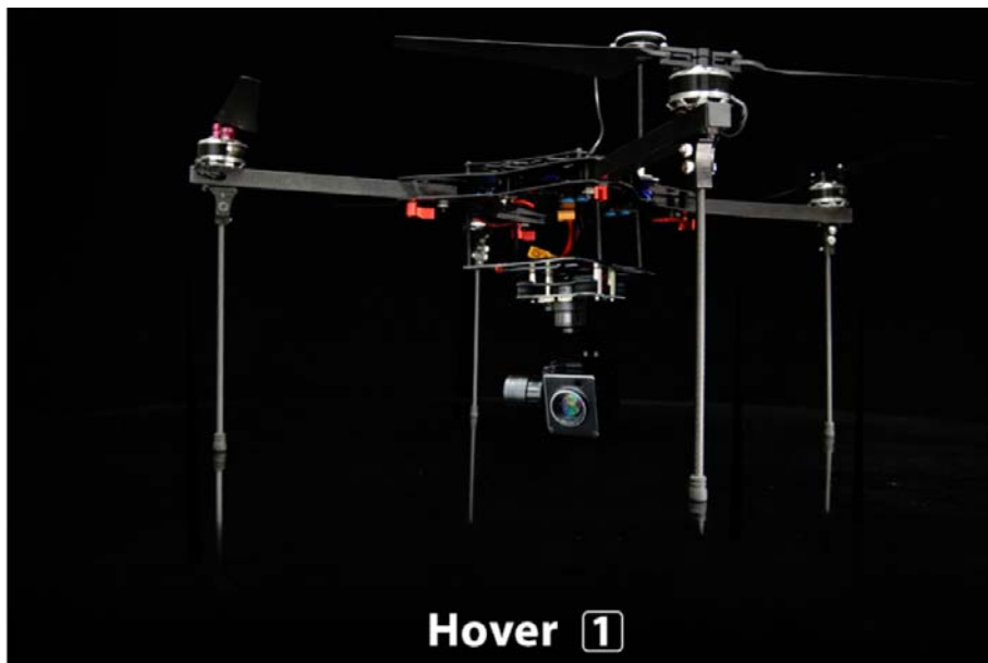
Figure 37. FH310Z Camera with Gimbal System Mounted on Foxtech Hover 1 Platform (Foxtech, 2017)
