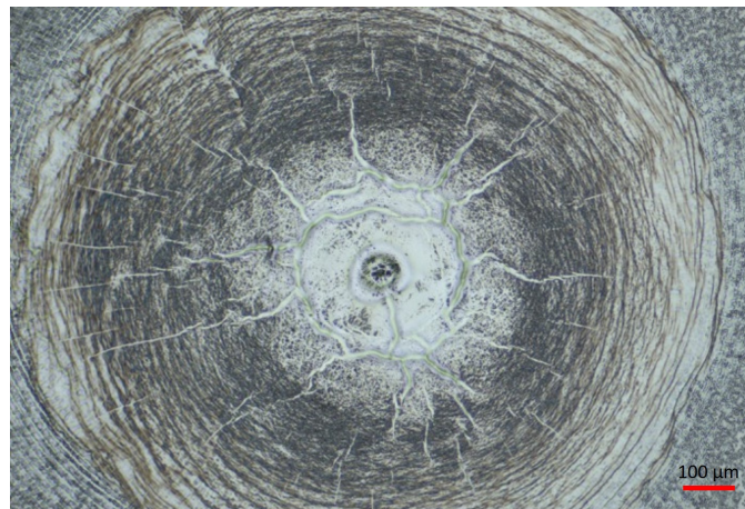
Figure 3. Structural cracks formed on InSb in the shielding regime. \lambda = 1064\ \text{nm} , \tau_p = 1\ \text{ns} , \omega_0 \approx 10\ \mu\text{m} , F \approx 3\ \text{kJ}/\text{cm}^2 , Material: InSb, P = 1\ \text{atm} , T = 300\ \text{K} .
