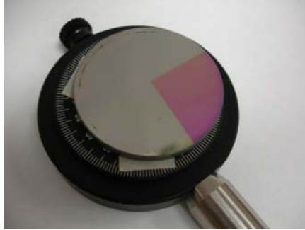
Figure 34. Ge sample showing the coating on the bottom right quadrant
