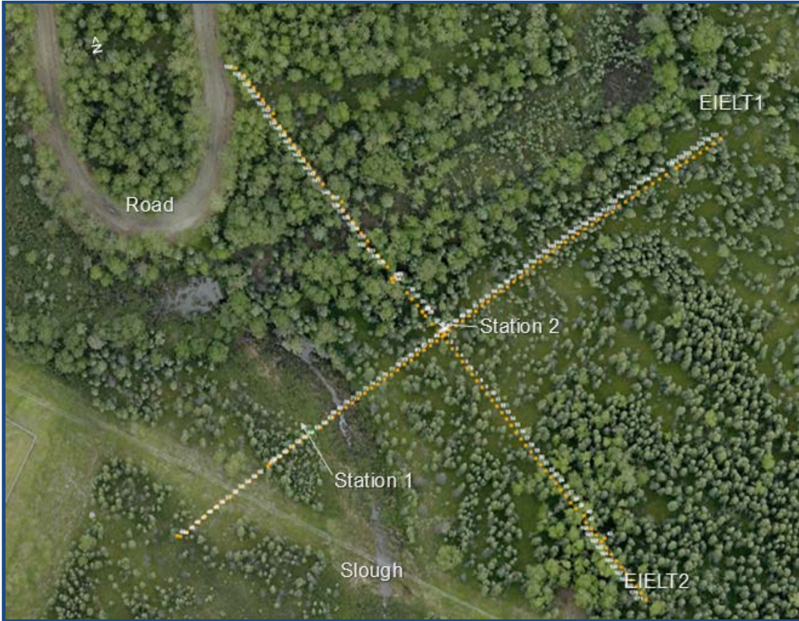
Figure 3.4: ERT and Frost Probe Survey Points [37]
