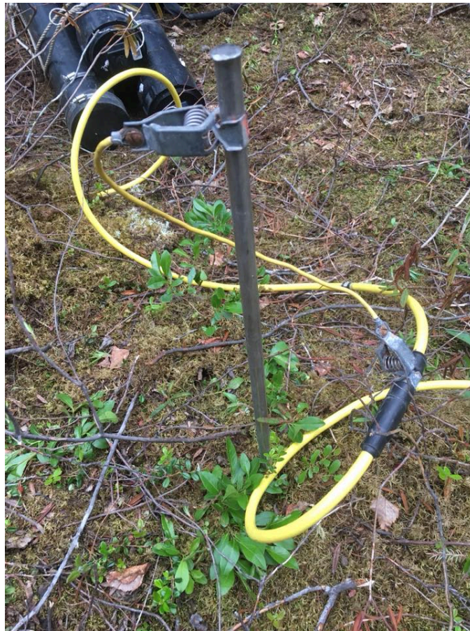
Figure 3.7: Standard ERT Probe Configuration
