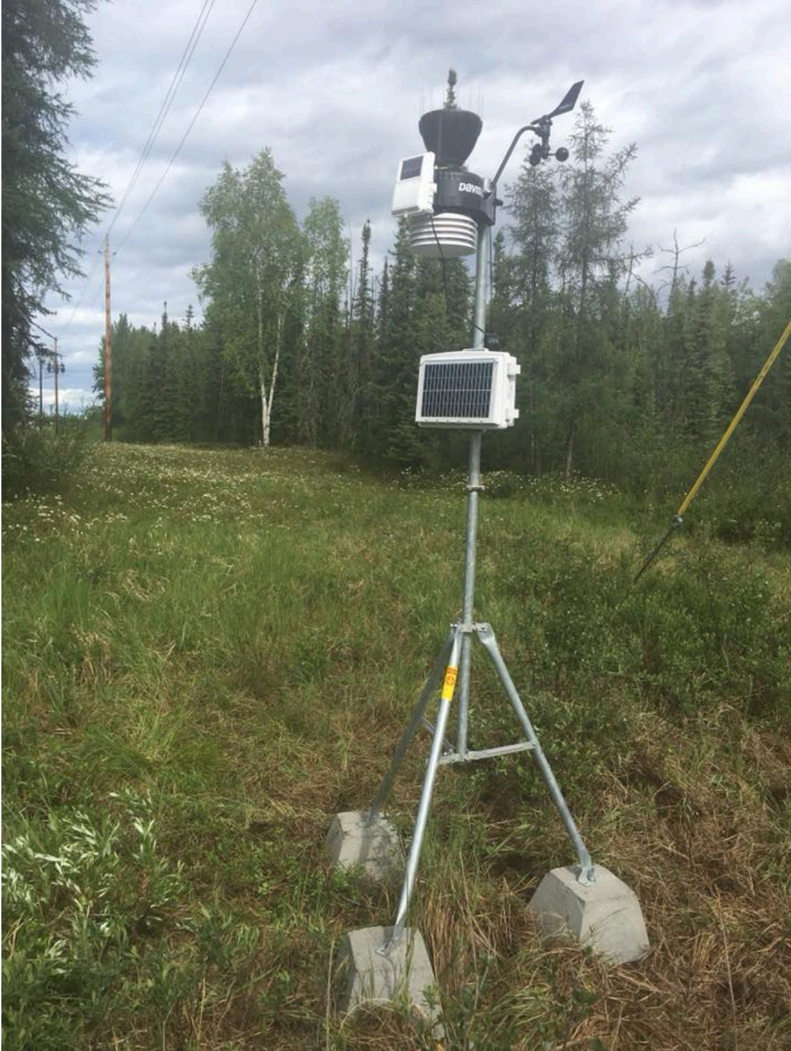
Figure 3.2: Weather Station Deployment and Orientation
