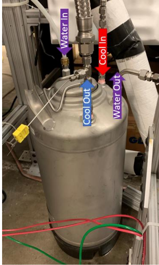
Figure 44: Water-cooling system for coolant line
