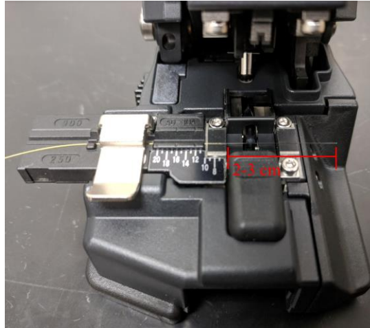
Figure 45. Sheathed Optical Fiber Positioned in the Cleaver
