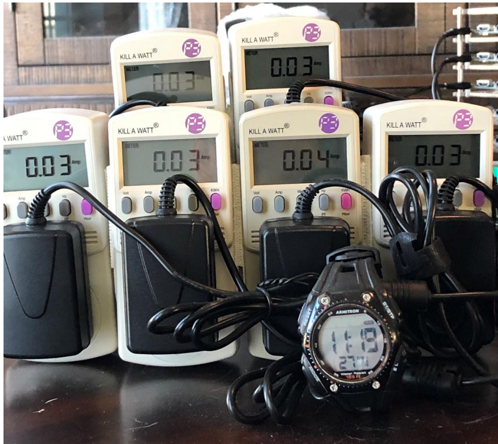
Figure 24. Kill-A-Watt Power Meters
