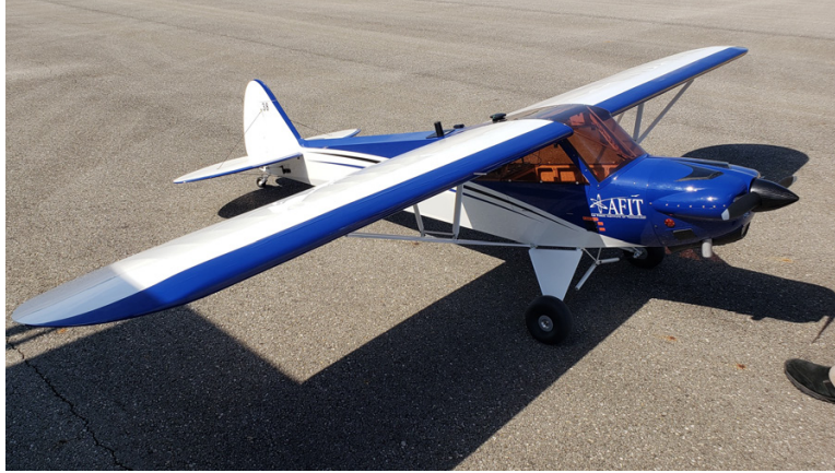
Figure 18. 40% scale Aeroworks Carbon-Cub survey aircraft
