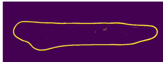
(d) The contour of the sample is extracted via binary adaptive and bitwise-NOT thresholds.
