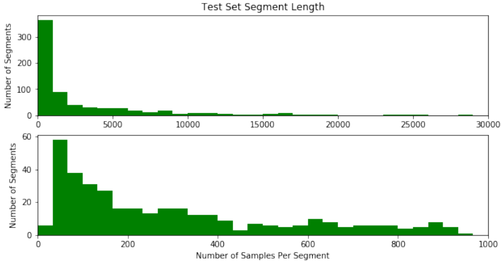
Figure 15. The top histogram shows the number of segments that fit into each range of the test set. The bottom histogram shows how the length of segments is distributed for segments under 1,000 samples in length. The bottom histogram is a detailed view of the first bar of the top histogram.
