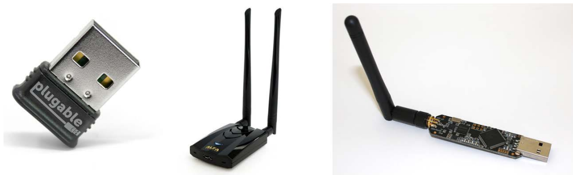
Figure 20. Scanning and Sniffing Equipment. Plugable Bluetooth adapter (left), Alfa AWUS036ACH Wi-Fi adapter (center), and Ubertooth One BLE sniffer (right)
