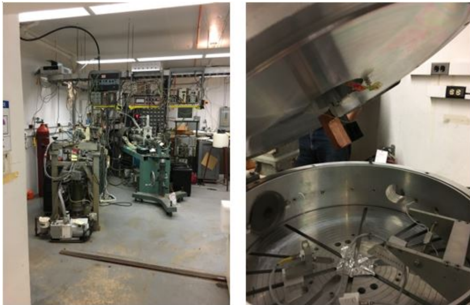
Figure 19. Edwards Accelerator beam line (left) used as the radiation source in this research. Its vacuum chamber (right) had a sample holder hanging on its lid; the sample was attached to a block of copper and its pin area (everywhere on the packaged sample but the actual sample area) was covered with conductive foam to prevent electrostatic charge buildup.
