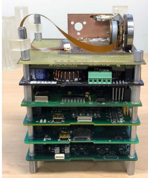
Figure 3.3. CubeSat PC/104 Payload stack [11]
