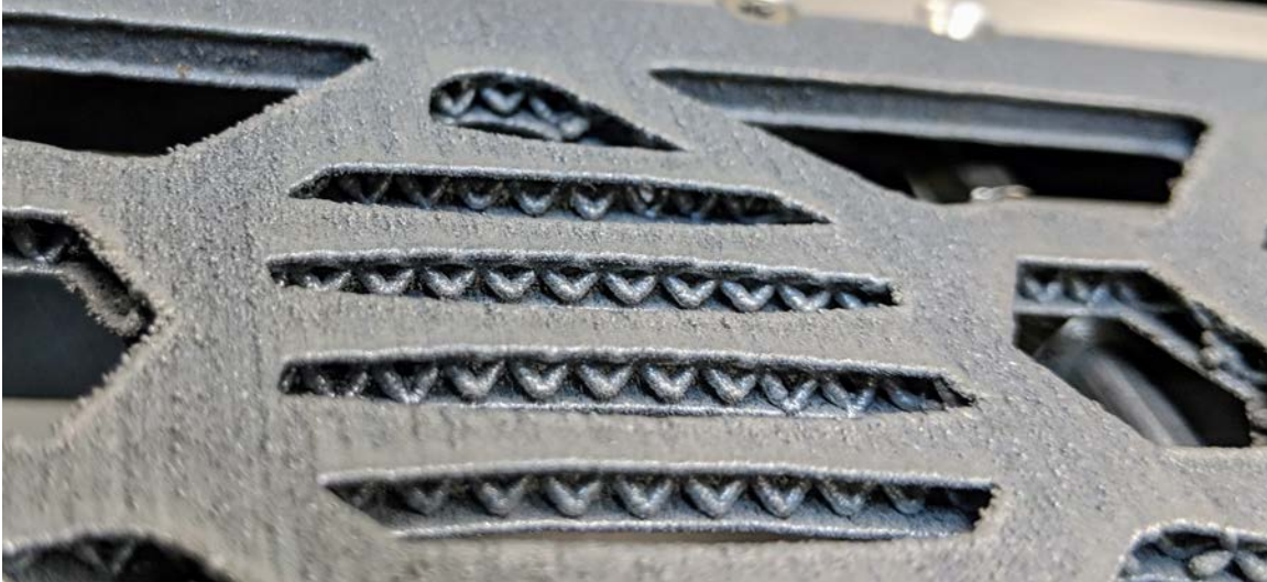
Figure 4.1. AlSi10Mg Lattice Based CubeSat Chassis [11]
