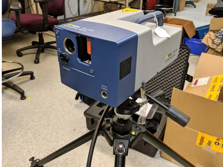
Figure 1.1. Polytec PSV-400 Scanning Vibrometer
