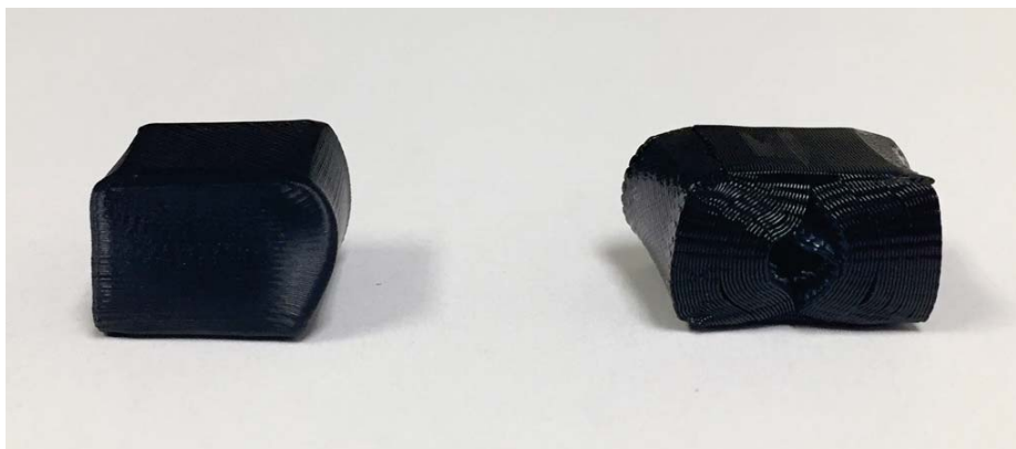
Figure 4.13. ZX compression specimen (left) and XY compression specimen (right).
