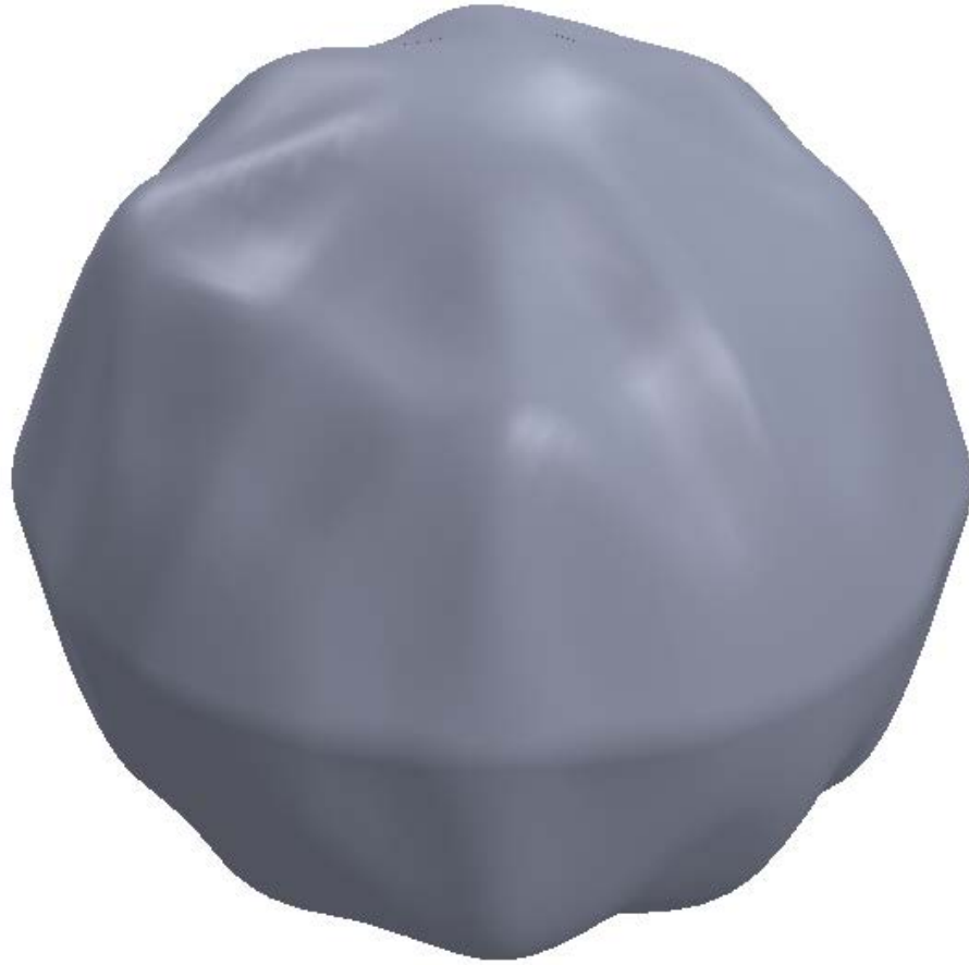
Figure III-9. Deformed VLTA V post conversion from structural analysis mesh to solid body
