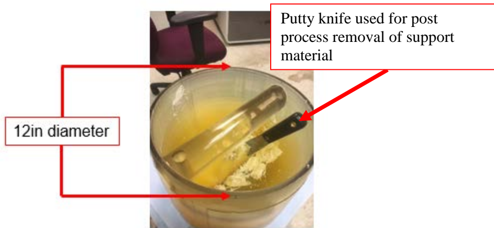
Figure III-13. Post processing of the bottom portion of the perfectly spherical model
