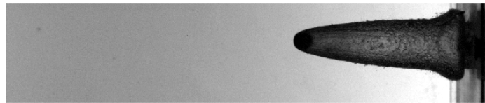
(b) Image taken at \Delta KE' of approximately 0.32 which corresponded to 1.60 ms after impact.
