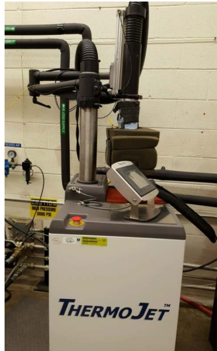
Figure 26. FTS ThermoJet ES for precision temperature cycles
