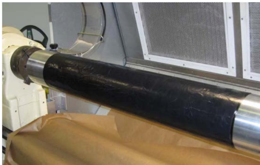
Figure 12. Preparation of support on Juno spacecraft [4] with outer layer CNT-sheet
