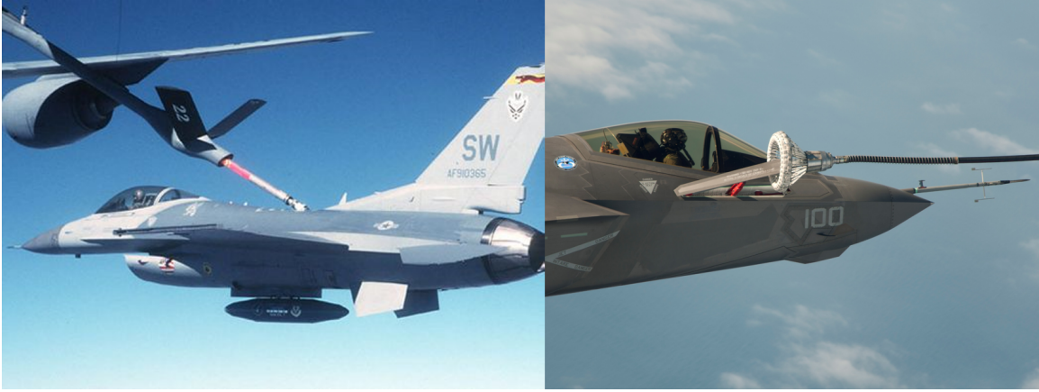
Figure 8. Comparison between Flying Boom (left) and Probe and Drogue (right) aerial refueling systems.
