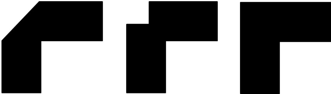
Figure 1. Examples of three common corner forms used in microstrip traces showing progressively worse performance, from left to right, are the fillet, step, and right angle corners [11].
