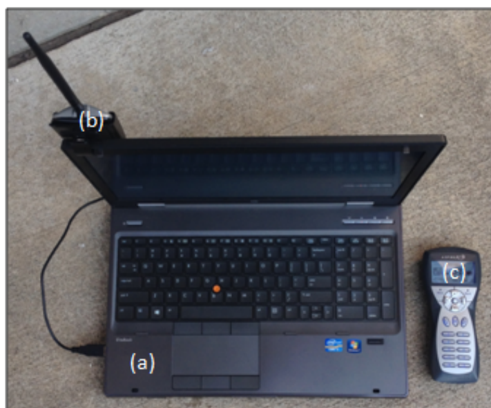
Figure 8. Equipment used for vulnerability scanning and exploitation: (a) HP Elitebook 8570w, (b) Alfa AWUS036H Card, and (c) Aspire RF Wireless controller [FR15a].
