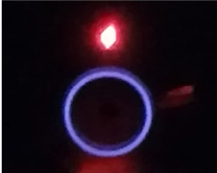
Figure 43: Thruster operating with new cathode mounting location
