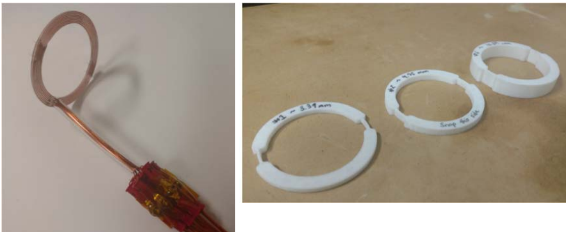
Figure 25: Magnetic sensor calibration ring and spacers
