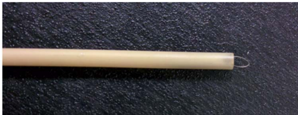
Figure 20: Emissive probe tungsten wire loop
