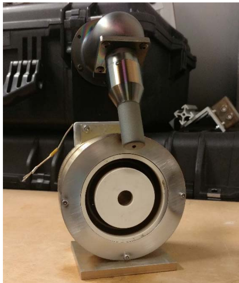
Figure 42: updated cathode mounting position
