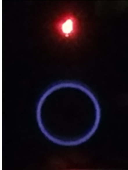
Figure 41: Thruster operating 20% above manufactures specified mass flow
