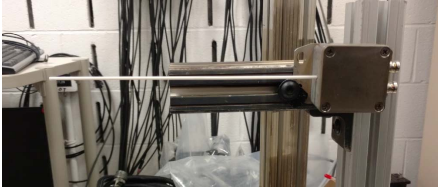
Figure 21: Fully assembled emissive probe
