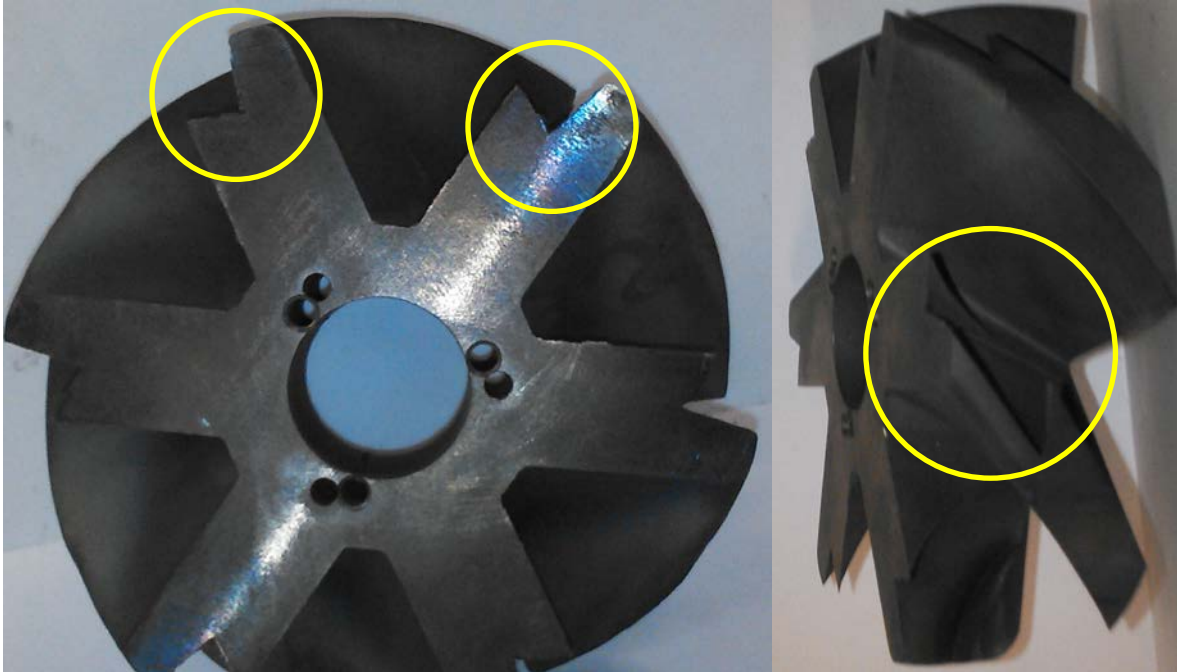
Figure 3.11: Final Low-Loss Hybrid Vane with RVC Channel Incorporated into Centerbody as Grown by Bastech Inc.
