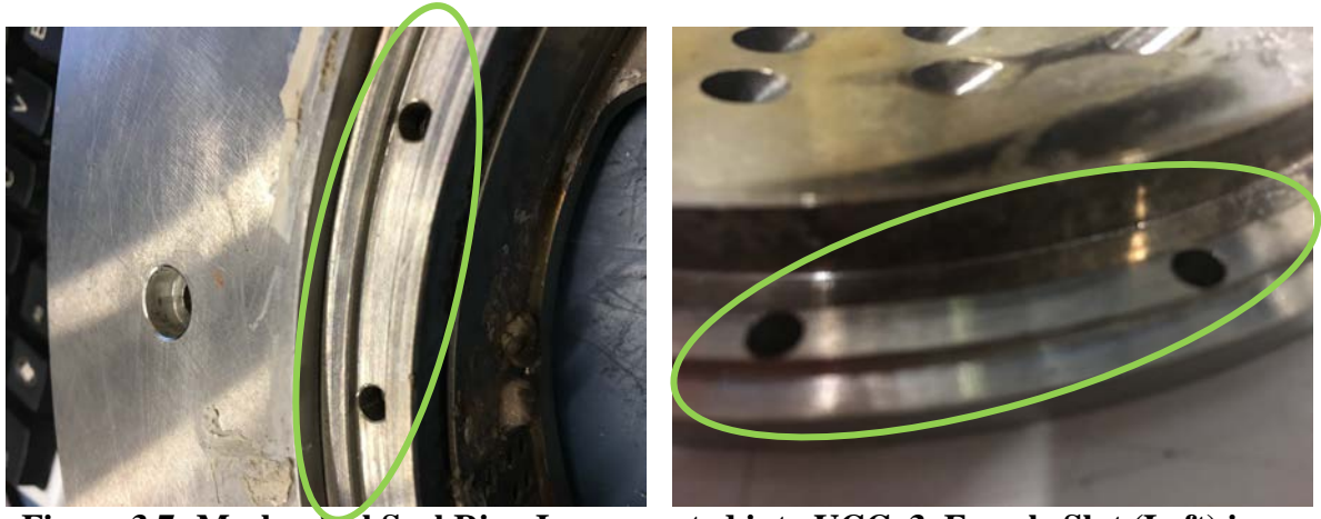
Figure 3.7: Mechanical Seal Ring Incorporated into UCCv3, Female Slot (Left) is on Outer Ring and Male Slot (Right) is on Driver Plate and Instrument Plate
