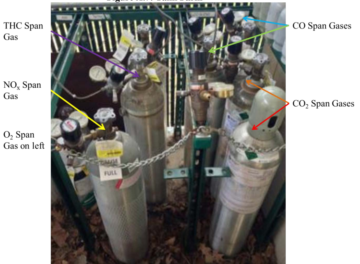
Figure A.8: Span gas tanks, O 2 , CO, CO 2
