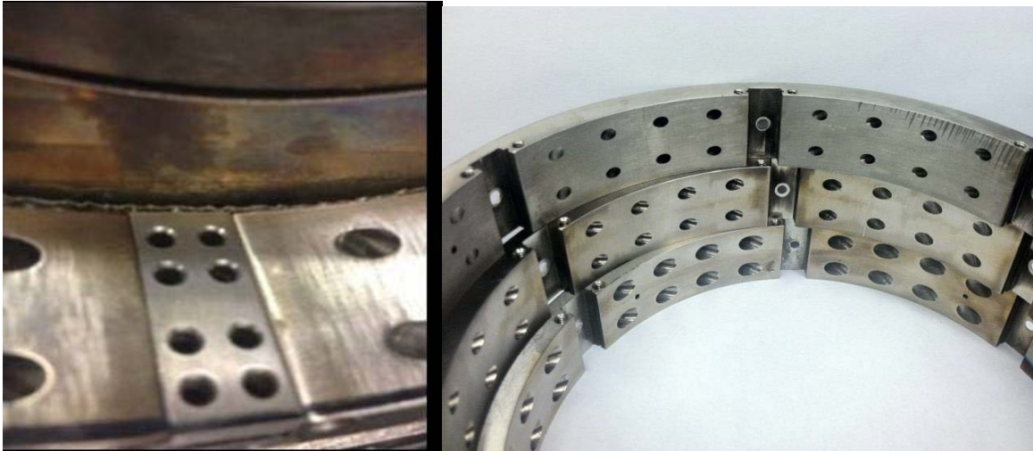
Figure 3.5: Close view of (left) Fuel Baffle Plate [37] and (right) side air injection holes for Discrete Air Source Configuration [25]
