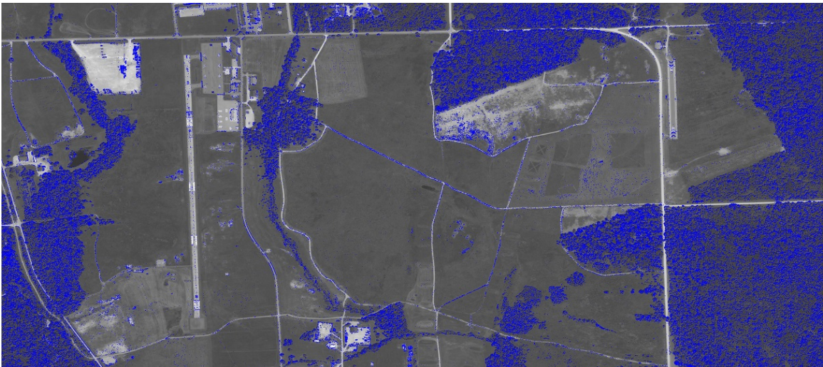
Figure 39. The database variant for the Sigma Parameter set at 0.8 instead of the base of 1.6. Feature locations are shown in blue.
