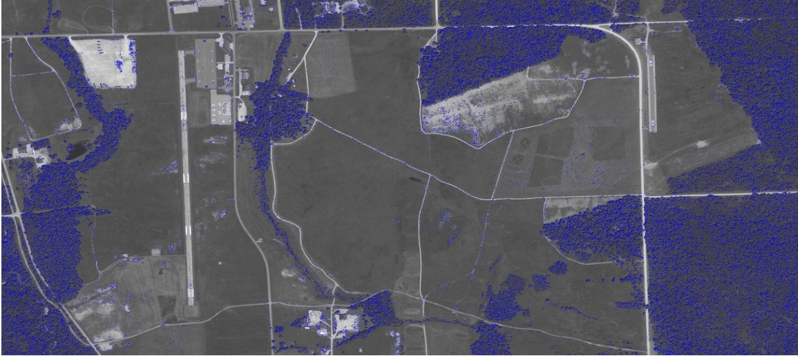
Figure 38. The database variant for the Edge Threshold set at 5 instead of the base of 10. Feature locations are shown in blue.
