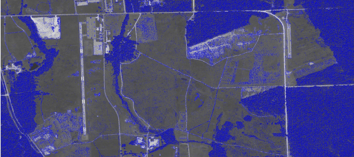
Figure 36. The database variant for the Contrast Threshold set at 0.02 instead of the base of 0.04. Feature locations are shown in blue.
