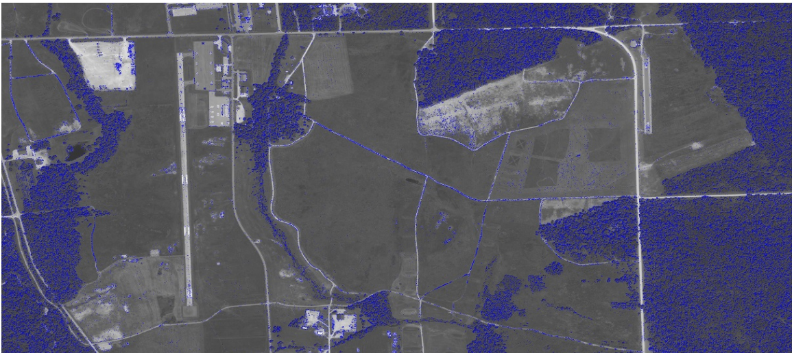
Figure 41. The database variant for the Edge Threshold set at 15 instead of the base of 10. Feature locations are shown in blue.
