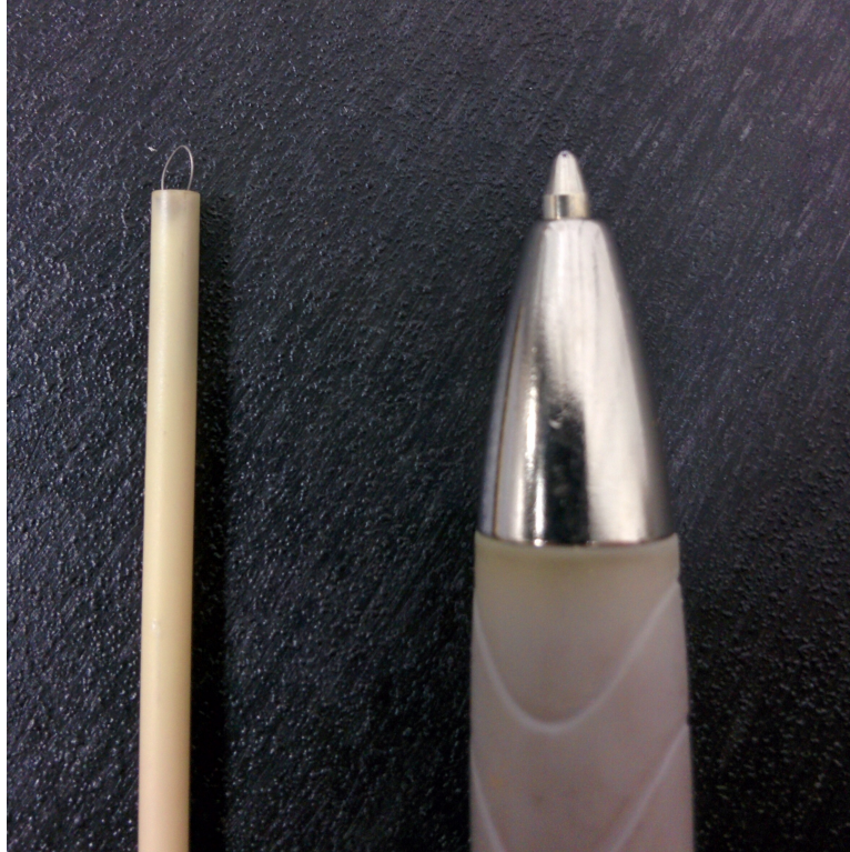
Figure 3.8: Emissive probe detail. Ballpoint pen for scale.
