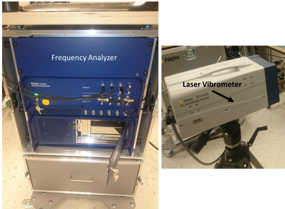
Figure 28: Polytec PSV-500 Laser Vibrometer Frequency Analysis System.
