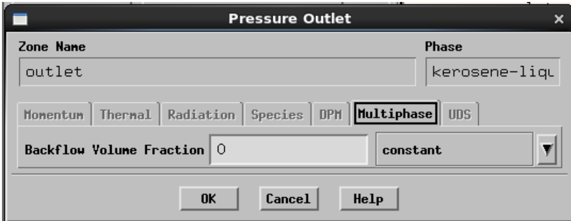
Figure 107. Fluent Settings: outlet multiphase settings (kerosene-liquid phase)
