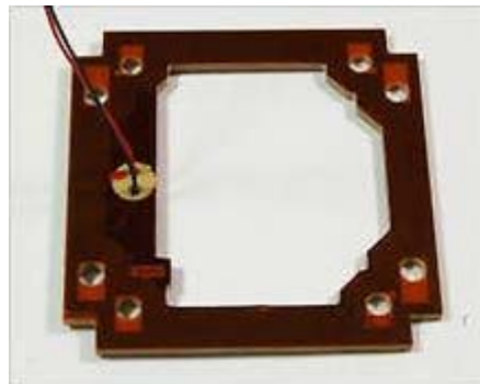
Figure 29 Clyde Space Z-Axis Magnetorquer [41]
