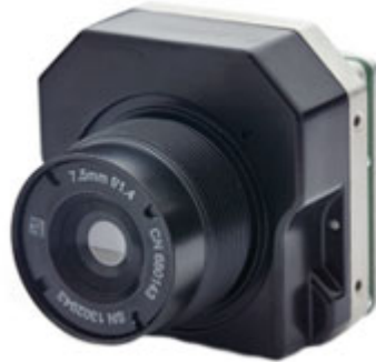
Figure 14 FLIR Tau 640 Uncooled Microbolometer [50]
