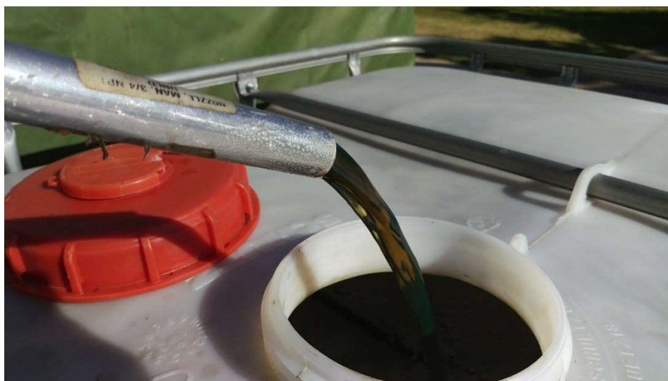
Figure 22 - Resulting Clean WMO from Cartridge Filter Rig
