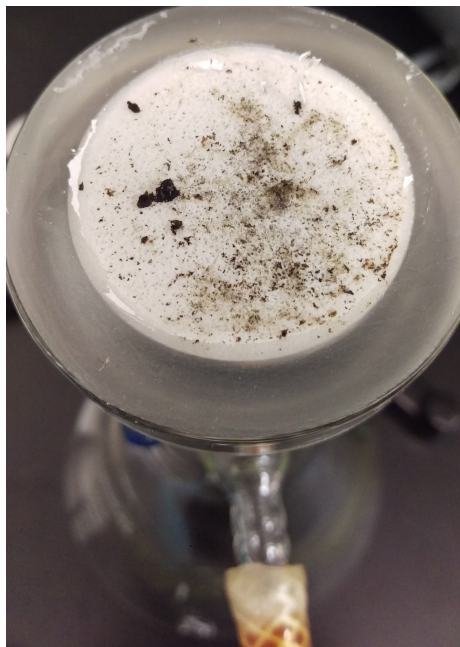
Figure 26 - Resulting Filter Media with Centrifuge Rotor Residual Particles
