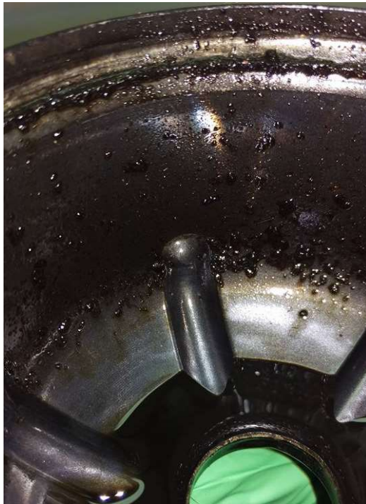
Figure 17 - Residual Particulate Matter in Centrifuge Rotor Cap
