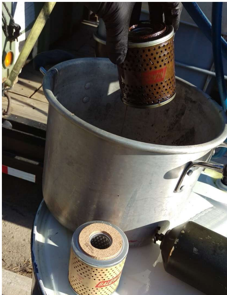
Figure 21 - Dirty Fuel/Water Separator Cartridge
