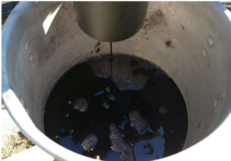
Figure 20 - Waste Drained from Clogged Fuel Filter
