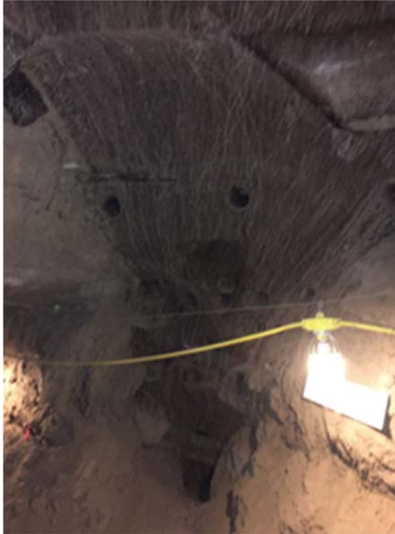
Figure 6: Ice Wedge Example in USACE CRREL Permafrost Tunnel in Fox, Alaska
