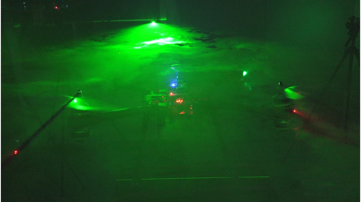
Figure 22. Complete Mixing after 6.06 seconds with Propellers On
