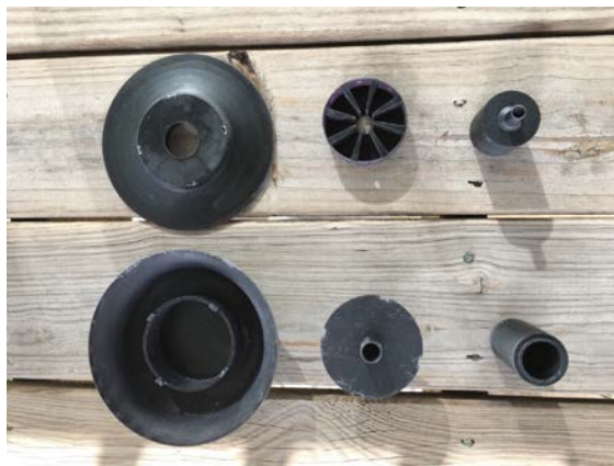
Figure 47. Exploded View of Six Component 3D Printed Inlet
