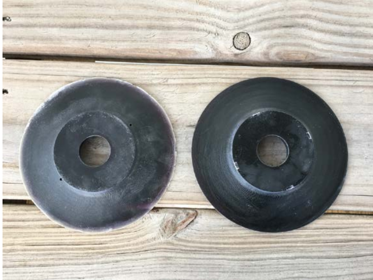
Figure 52. Side-by-side comparison of initial design (left) and revised design (right) of Fan Plate
