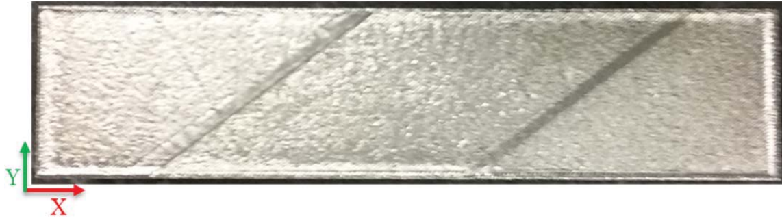
Figure 38. Sample L-41 top surface, visible diagonal striations on top surface due to beam pattern variation.
