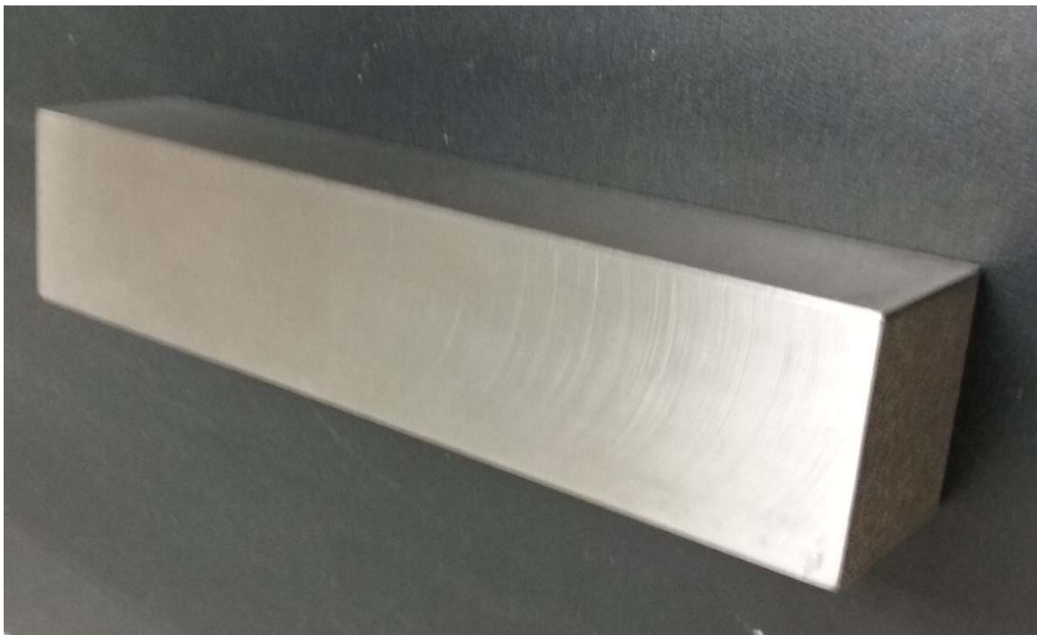
Figure 27. Sample B-41 top and side surfaces post machining, tooling marks visible on both surfaces
