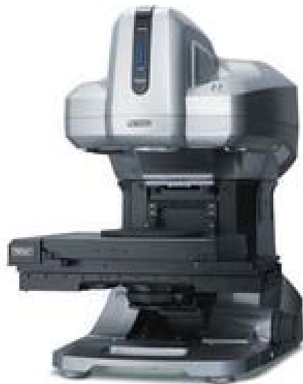
Figure 18. 3-D Measuring macroscopic, Keyence Model VR-3200
