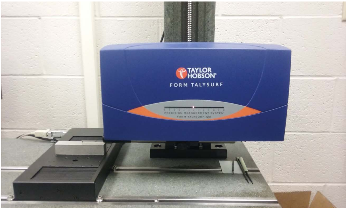
Figure 17. Profilometer set-up, used to generate 3-D surface roughness measurements
