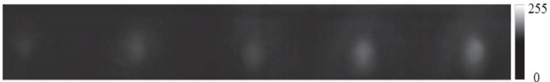
Figure 31. Combine data from 11 center matrices compiled into C-Scan, 5 MHz
