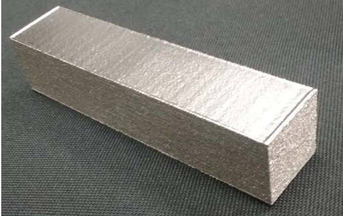
Figure 26. Sample B-41 top and side surfaces prior to machining.
