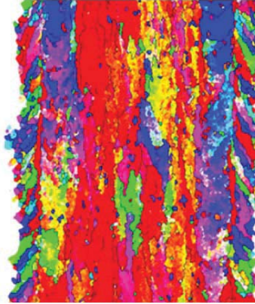
Figure 45. Electron Back Scatter (EBSD) map from X-Z cross sections [25]
