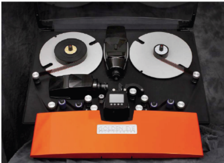
Figure 7. The Goldeneye scanner that is used by LLNL to digitize the NUDET films [30].
