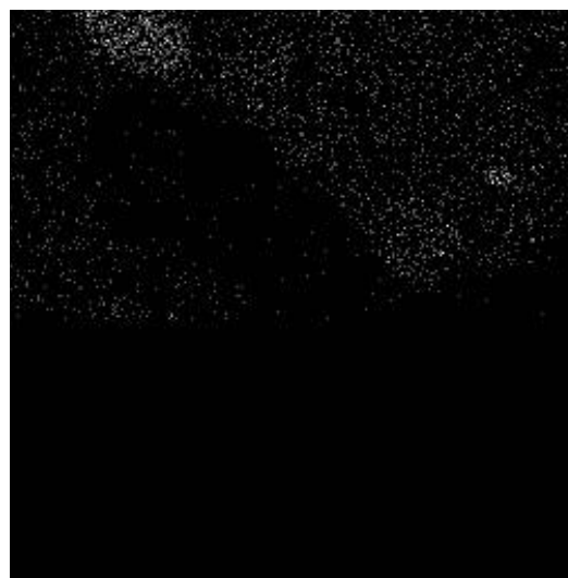
Figure 59. The 1% concentration of Sn is shown evenly distributed throughout the crystal. The response as seen in the image is not as intense as seen for Cs in Figure 57. This is expected as it occurs only 1% of the time in the matrix.
