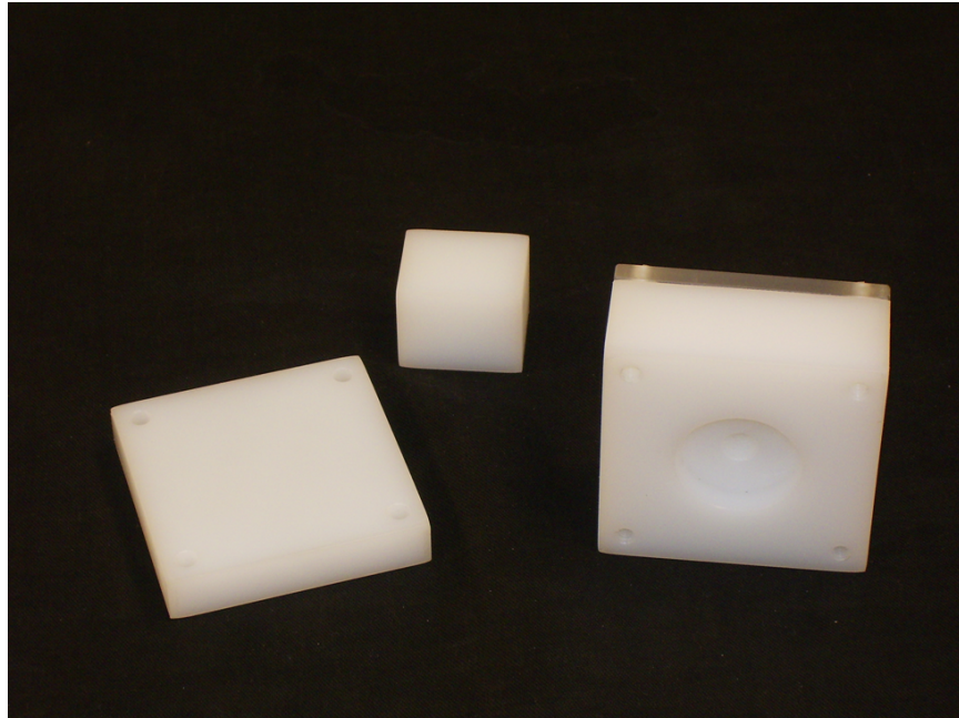
Figure 51. The customized plastic mount made it easier to change samples and isotope planchette sources. The planchette source holder on the right had a bore down the middle to reduce gamma ray attenuation. If an irregular target sample was used the center block in the frame was used to hold the source in the path of the gammas coming from the bore. Although efficiency was lost due to solid angle losses the consistency of results improved. The mounting scheme worked well for the wafer-like shape of the \text{CsI}(\text{CdI}_2) samples as demonstrated in Figure ??.
