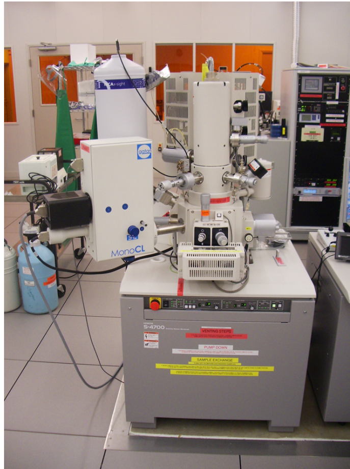
Figure 18. The SEM is capable of providing 500,000 times magnification for sample imaging. The CL apparatus is on the left side of the image labeled monoCL made by Gatan. A set of computers to the right of the instrument run the SEM and the Gatan CL instrument separately.
