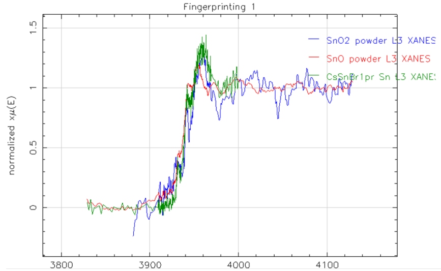
Figure 28. The CsBr:Sn-1\% EXAFS data is plotted with SnO^{2+} and SnO_2^{4+} powder data. As discussed previously, EXAFS interactions are element specific. Thus the chemical interactions of the oxygen, cesium and bromine atoms, respectively, do not contribute to the shift in the XANES structure. The shift is due to the lack of two electrons as compared with Sn^{2+} . The CsBr:Sn-1\% with the Sn^{2+} configuration has been studied in previous literature [Savchyn et al., 2007]. Thus it is easy to deduce the oxidation of the Sn^{4+} oxidation in the CsBr:Sn-1\% samples.
