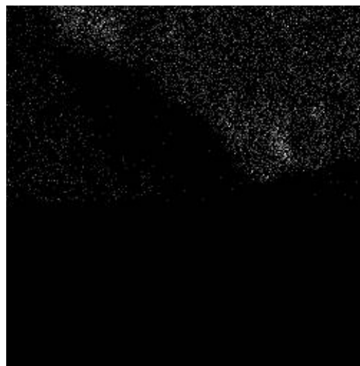
Figure 58. The Ca shows up very rarely in the crystal. The minimum concentration to register for XRF is just below 1%. Despite Ca not showing up in the analysis report it is present in the crystal.
