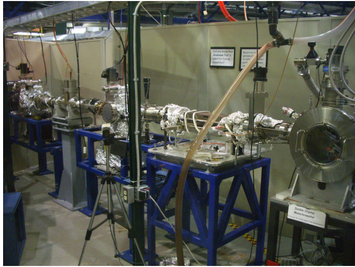
Figure 15. The DCM line is the x-ray line used for EXAFS, XANES and other x-ray absorption analysis techniques. The double monochromator can be seen on the right side of the image. X-rays exit the synchrotron at various wavelengths. A monochromator is used to tune the x-rays to the desired energy, or I_o . The entire line is kept under vacuum to reduce x-ray interactions with air or other molecules before they hit the samples. The tin foil is used to retain heat during beam line "baking". The separate lines at CAMD are baked intermittently to help release molecules that build up in the lines. Any liberated molecules are quickly expelled in the vacuum process.
