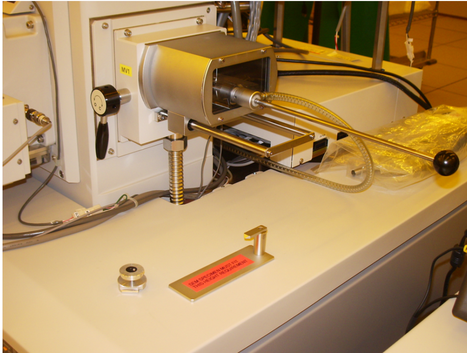
Figure 20. The sample exchange chamber is where a vacuum is drawn on the sample and then inserted into the SEM chamber via the pushrod seen protruding from the chamber. The sample pedestal is seen in the foreground with a measuring standard. The entire height of the sample and pedestal must be less than 1-inch to fit under the monoCL mirror for CL analysis. Otherwise, damage can occur to the mirror when it is brought into position for analysis.
