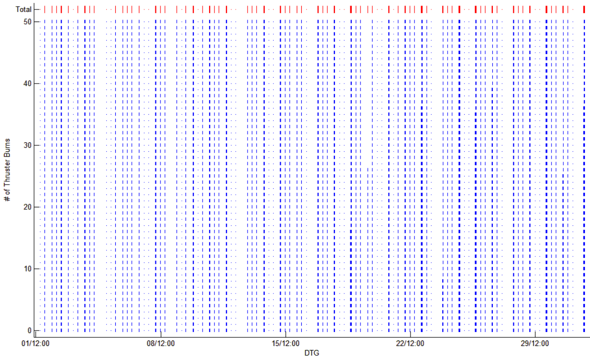
Figure 4.42 Target Access Bands for 30 Day Period at 40 deg Inclination Using Thruster 1 (Thrusting Anti-Normal then Normal)
