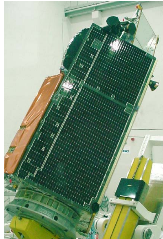
Cryosat with star trackers and baffles
