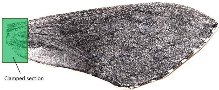
Figure 25: Paper wing used in frequency experiments.
