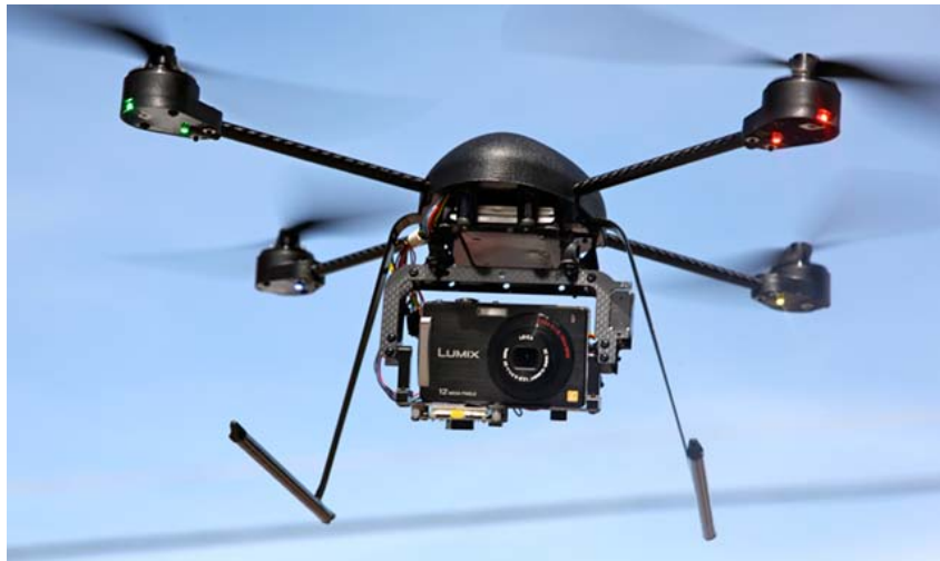
Figure 3: The D raganFlyer X6 co mmercial U AV with a h igh-resolution (1080p) camera, has an 85 cm span [3].
