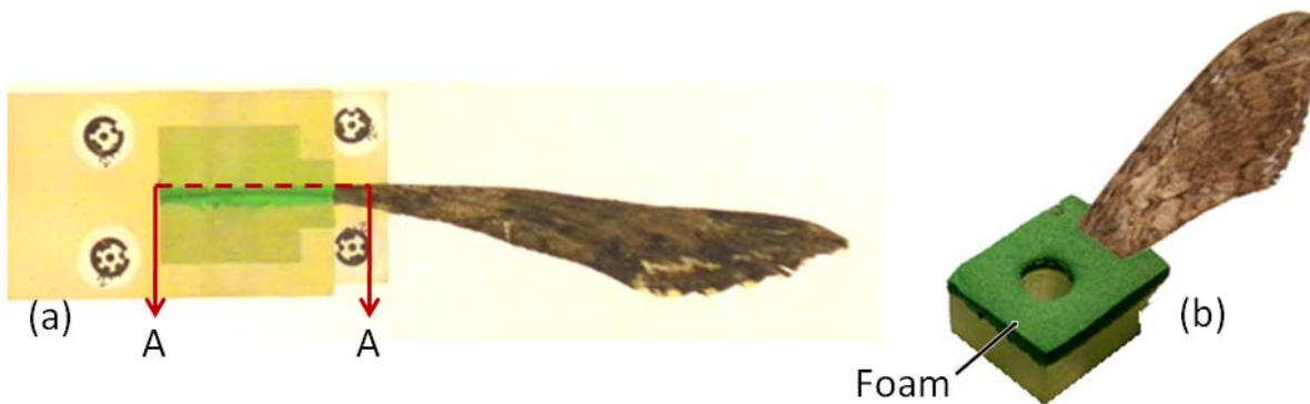
Figure 12: Side view of a clamped Manduca Sexta forewing (a), and the foam-lined clamp of cross-section A-A (b). The four symbols shown in (a) are reference points for future photo-modeling use.
