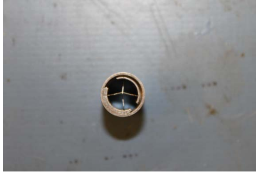
Figure 31 Sample torsional spring used in the balance
