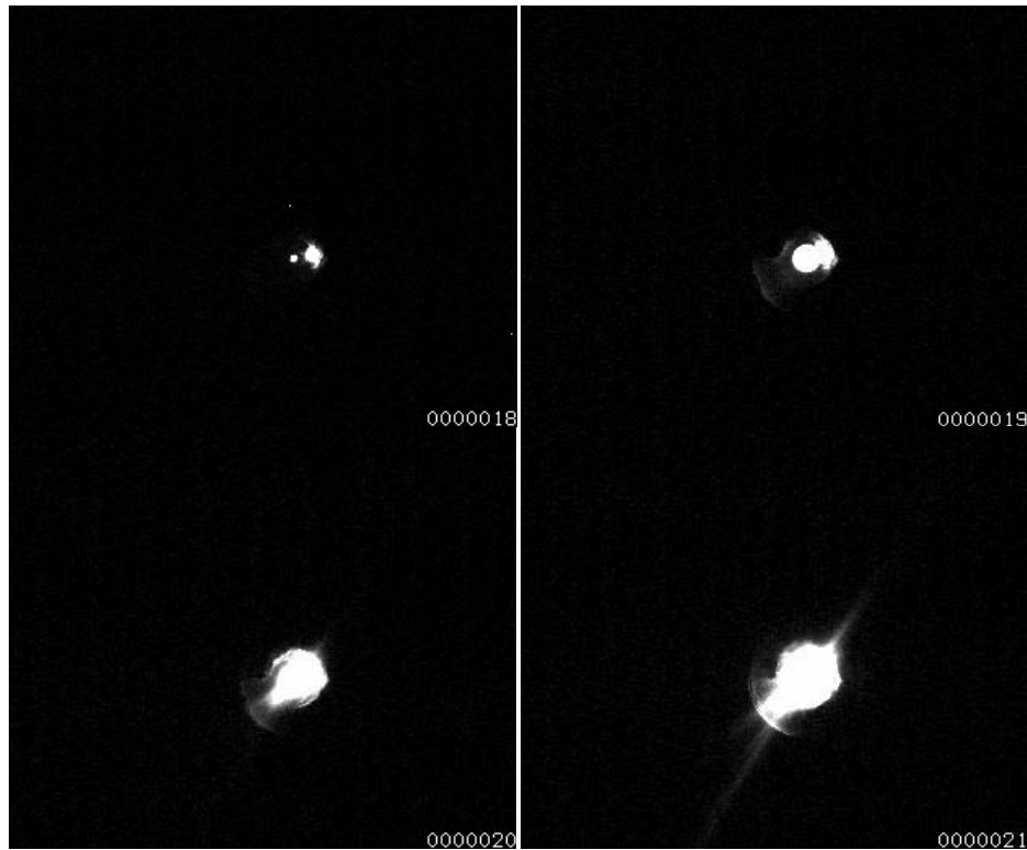
Figure 69 Spark Formation on Mass Collection Thruster
