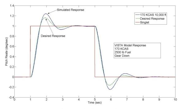
Figure 35: Approach Configuration Step Response
