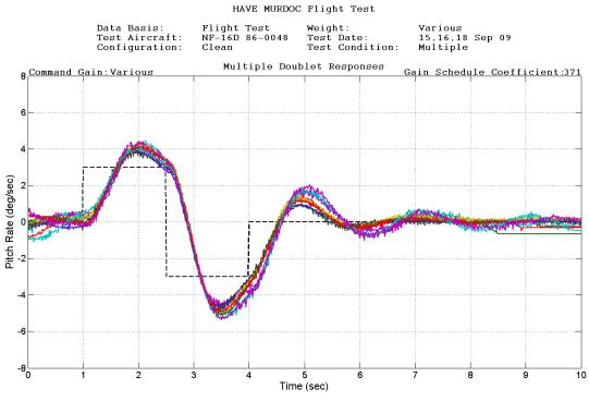
Figure 86: Doublet (Multiple Conditions)
