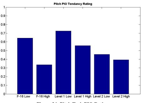
The normalized PIO ratings for the pitch tasks are shown in Figure 24.
