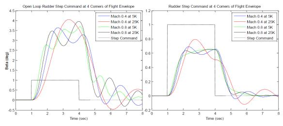
Figure 15: Open and Closed Loop Rudder Step Response
