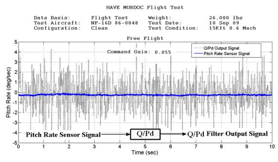
Figure 37: Pitch Rate Sensor Noise Amplification
