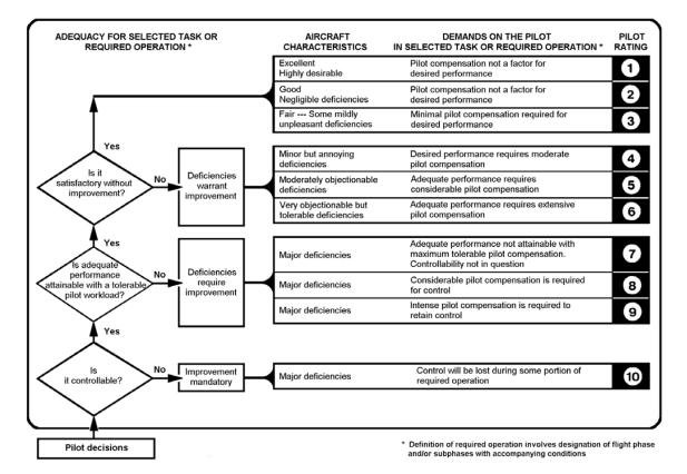
Figure 2: Cooper-Harper Rating Scale [Cooper and Harper, 1989]
