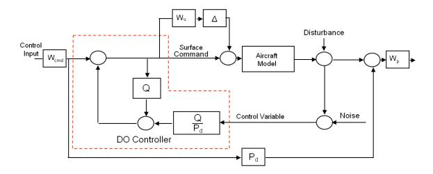
**Figure 8: Weighted Disturbance Observer Model**
