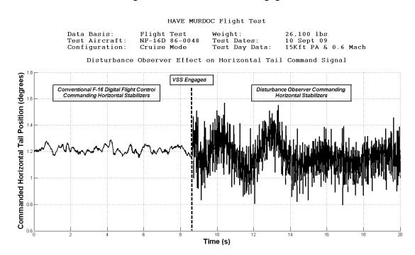
Figure 36: Horizontal Tail Command Signal
