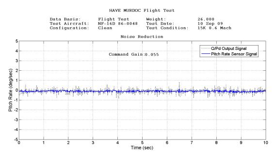
Figure 38: Reduced Noise with New Q Parameters
