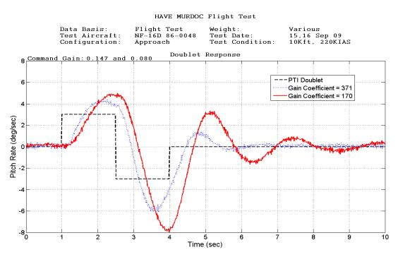
Figure 43: PTI Doublet Comparison between  $k_{cmd}$  = 37.1 and 17.0
