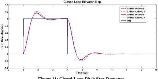
**Figure 11: Closed Loop Pitch Step Response**
