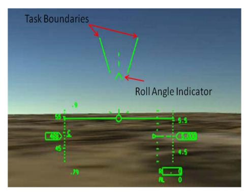
Figure 22: Roll Tracking Task HUD Display
