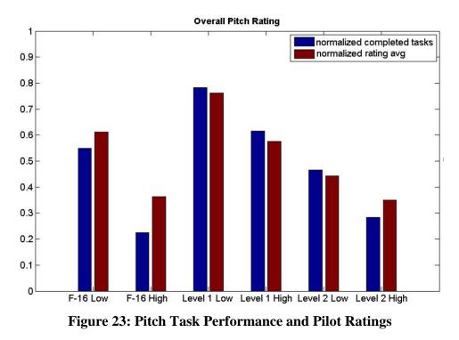
It is clear that the controller ratings fell in line with task performance, which is a result that can be expected due to the fact that the pilots normally associate performance with quality of handling. Next, it is clear that the low altitude, high speed condition performed and rated better than the high altitude, slow speed condition for all controllers. Finally, the level 1 DO controller rated and performed the best with the level 2/3 DO rating and performing the worst.
