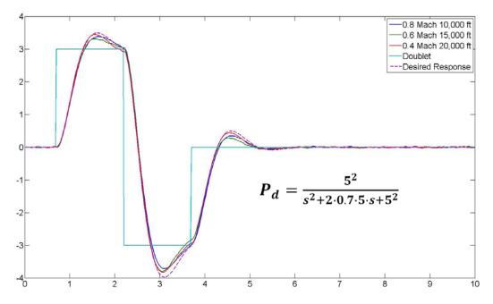
Figure 49: Doublet Response with New Desired Dynamics
