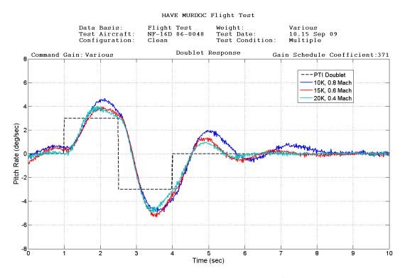
Figure 42: PTI Response at Three Flight Conditions
