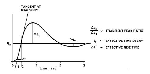
Figure 7: Pitch Rate Response to a Step Input
