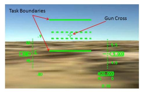
Figure 21: Pitch Tracking Task HUD Display
