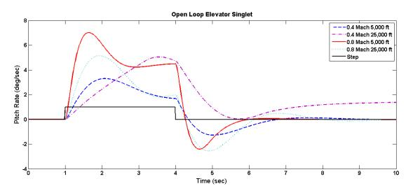
Figure 10: Open Loop Pitch Step Response
