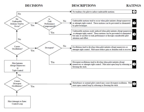
Figure 3: Pilot-in-the-loop Oscillation Rating Scale
