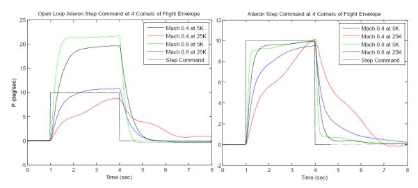
Figure 12: Open and Closed Loop Roll Step Response
