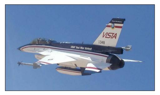
Figure 27: Variable stability In-flight Simulator and Test Aircraft (VISTA)
