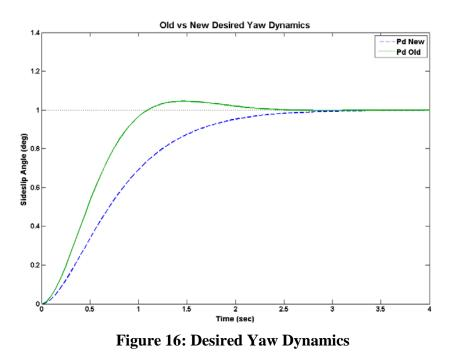
After changing the desired dynamics, the design filter parameters were adjusted to maintain performance. The values chosen were  $\omega_{Q_yaw} = 50$  (rad/sec) and  $\zeta_{Q_yaw} = 0.9$ . Changing the desired yaw dynamics resulted in the following closed loop response to a rudder step (Figure 17).
