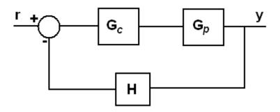
Figure 5: Typical Feedback Control Diagram
