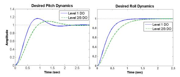
Figure 20: Desired Pitch and Roll Dynamics (Level 1 & Level2/3)
