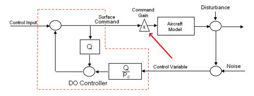
Figure 18: DO with Command Gain Applied
