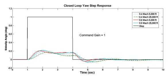
Figure 17: Closed Loop Response to a Rudder Step
