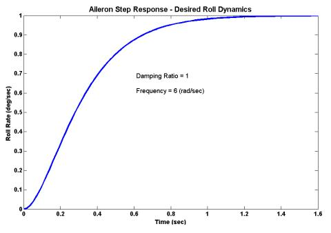
Figure 13: Second Order Desired Roll Dynamics
