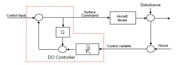
**Figure 6: Disturbance Observer Architecture**
