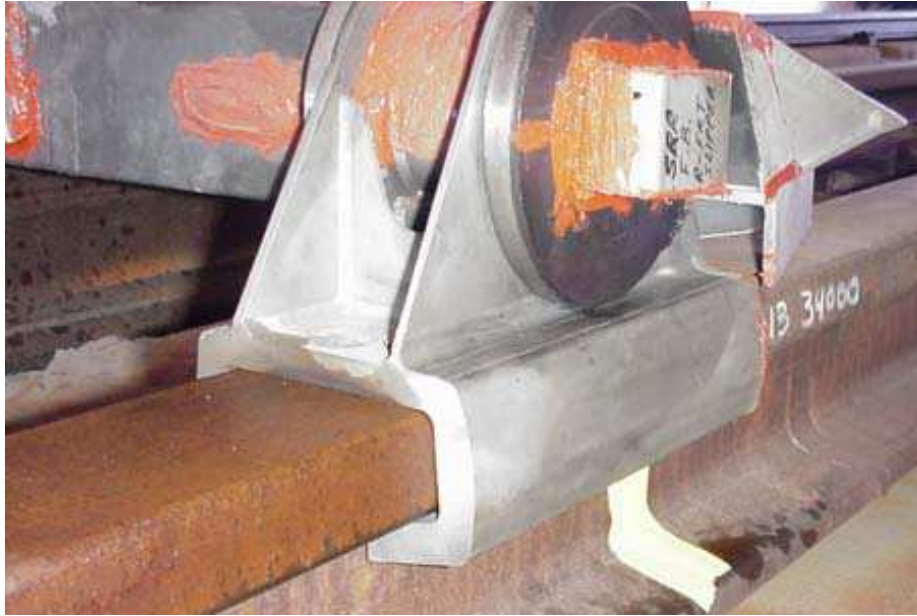
Figure 1.4: Slipper Configuration for High Velocity Sleds
