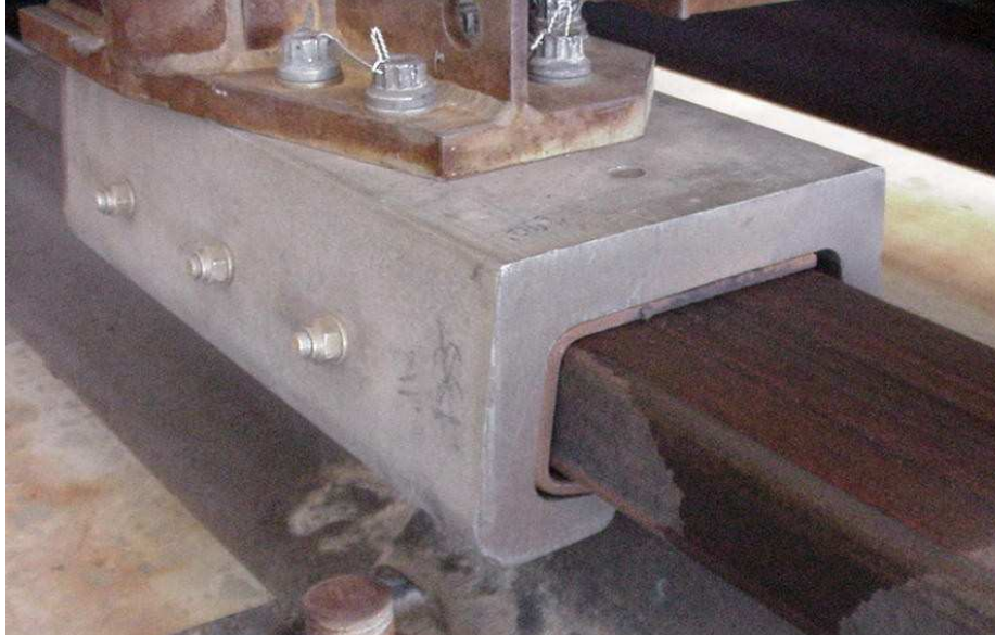
Figure 1.3: Slipper Configuration for Low Velocity Sleds
