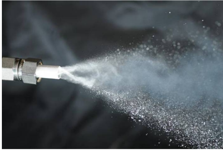
Figure 4.4: Characteristic profile of particles exiting a mixing shroud tube.
