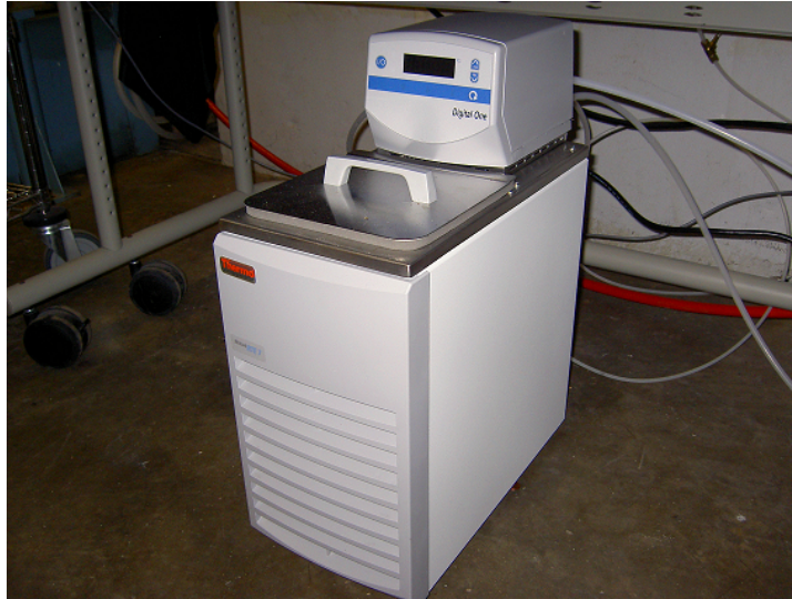
Figure 3.4: Refrigerated bath filled with deionized, distilled water for heat exchange.
