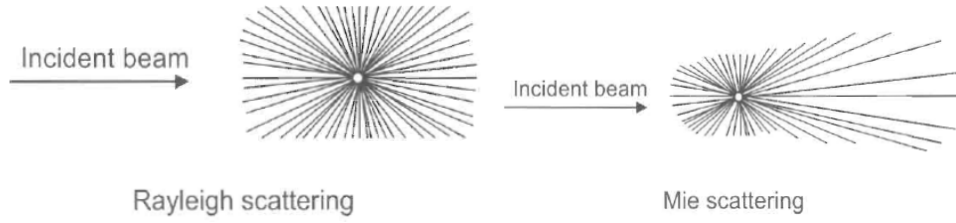
Figure 2.2: Rayleigh and Mie scattering characteristics. [12]
