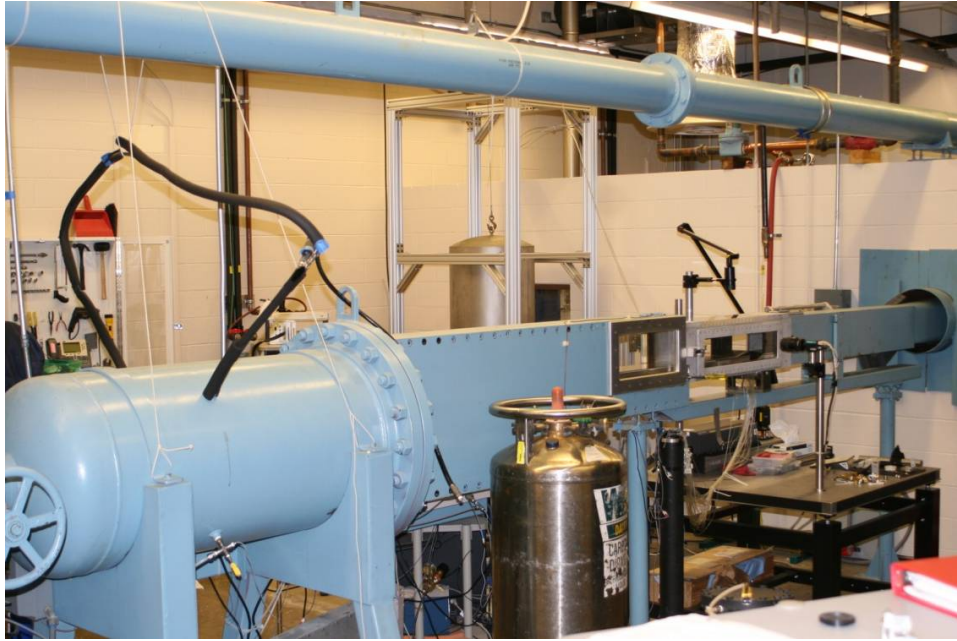
Figure 3.5: AFIT 6 inch by 6.5 inch supersonic blowdown wind tunnel.
