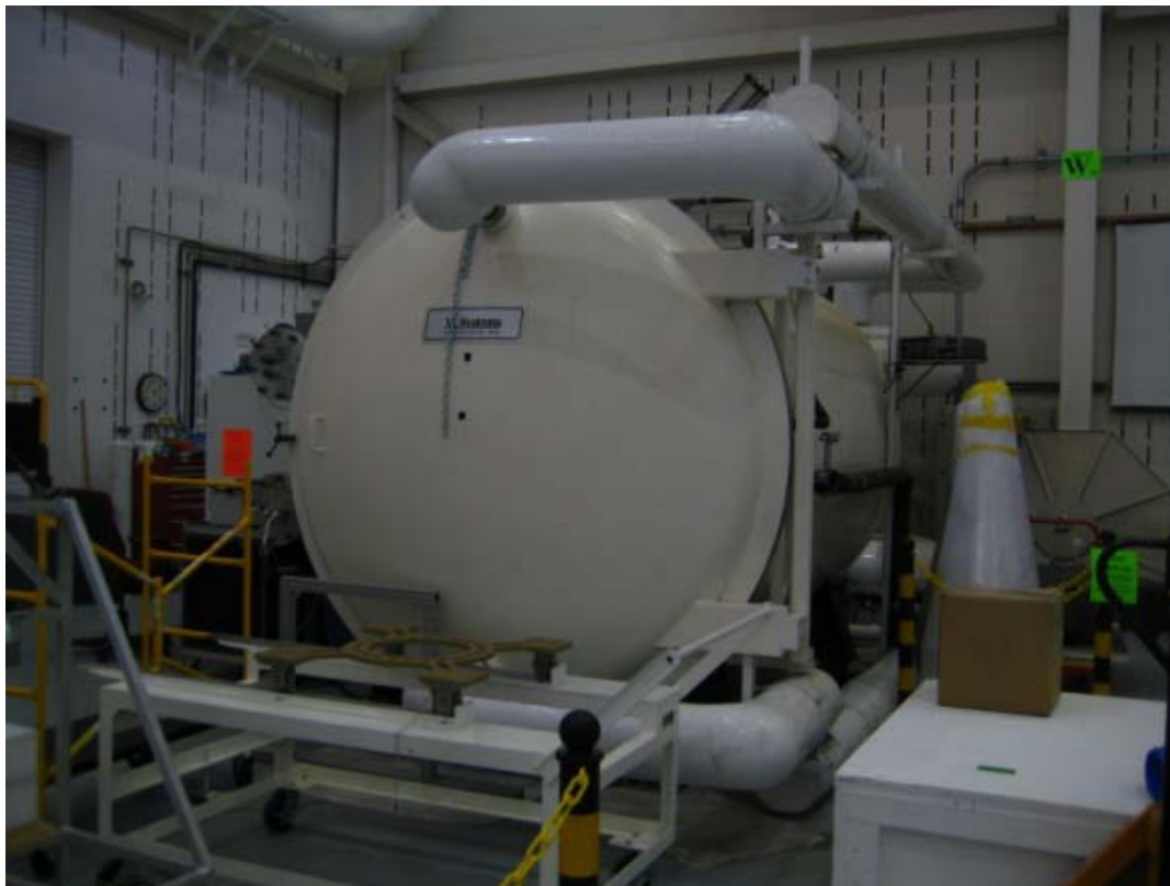
Figure 29. AEF Thermal Vacuum Chamber
