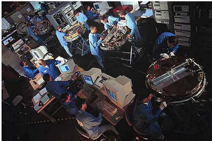
Figure 18. Manufacture of Multiple ORBCOMM Satellites in Parallel [19]
