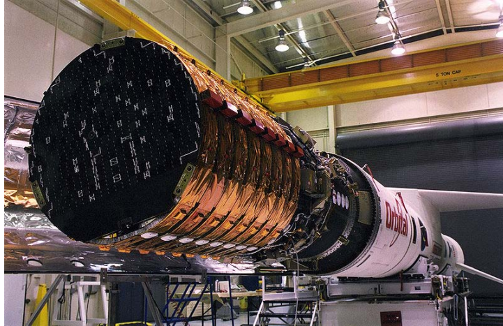
Figure 17. ORBCOMM Satellites in Pegasus Launch Vehicle Integration [19]
