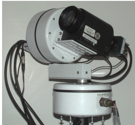
Figure 3.3: A camera subsystem consists of a two axis gimbal, zoom-focus lens, a high speed camera, and controller computer (not shown).
