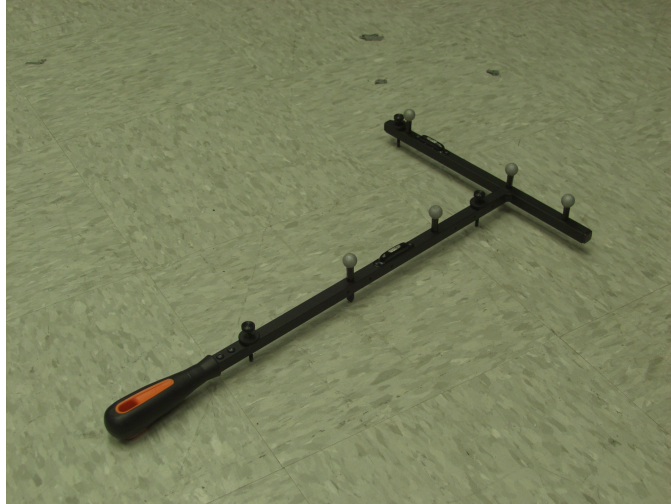
Figure 3.5: Calibration wand used to calibrate and set the origin of the videogrammetry system
