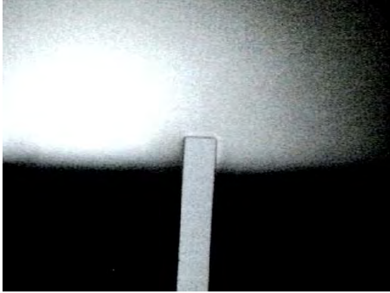
Figure 5.5: Top view from the microscope built into the nanoindenter. This is the view used when using the micrometer and vertical stage in setting up the alignment before the experimental runs. Note that the strike plate is out of focus because it is below the cantilever.
