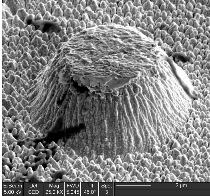
Figure 8.5: Gold coated bump (0602-1.12(D)) after adhesive failure at 20,000 cycles.
