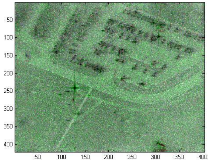
Figure 4.23: This is the same SAR image on Figure 4.22 but computed for CMY color space. The process of compute the CMY color space image is by subtracting the RGB values of Figure 4.22 from one.
