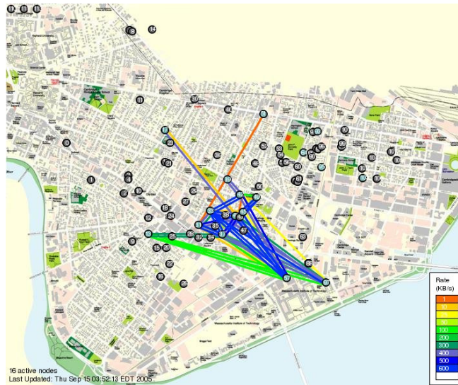
Figure 2-5. Grid/Roofnets Link Map of MIT with nodes and link data rate
